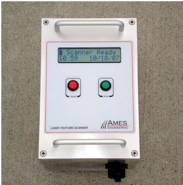
Figure 3.19: Laser Texture Scanner and an example of surface texture profile it measured (Section 655HB, #4P mix with PG 76-22PM binder). (Photo of LTS courtesy of Ames Engineering, Inc.)
