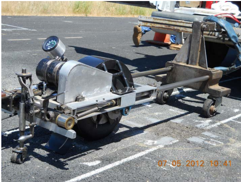
Figure 3.21: California Portable Skid Tester (CST) used to measured surface skid resistance following California Test (CT) 342.
