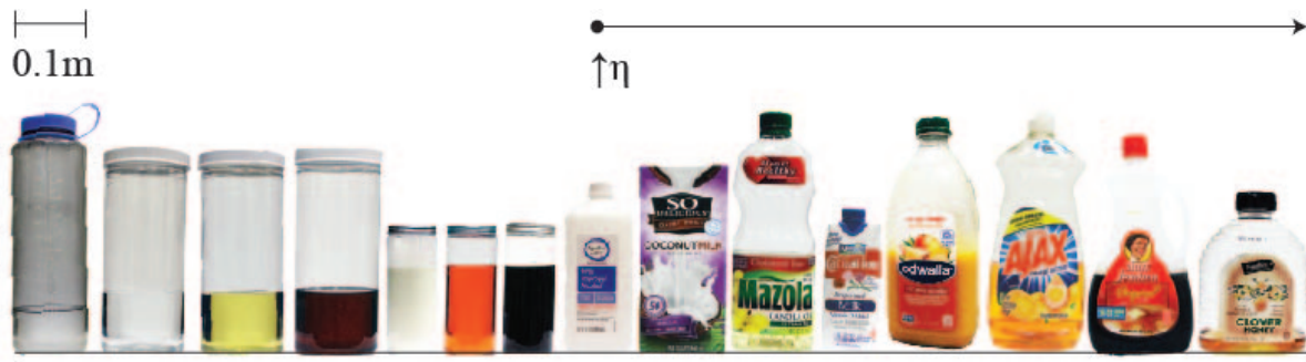
Figure 2.3: From left to right: 48oz Nalgene water bottle used in exploratory analysis, 3 large cylindrical containers used in viscosity estimations, 3 small cylindrical containers used in all experiments, and isopropyl alcohol, coconut milk, canola oil, evaporated milk, mango juice, dish soap, syrup, and honey, arranged in order of approximately increasing viscosity. © 2019 IEEE
