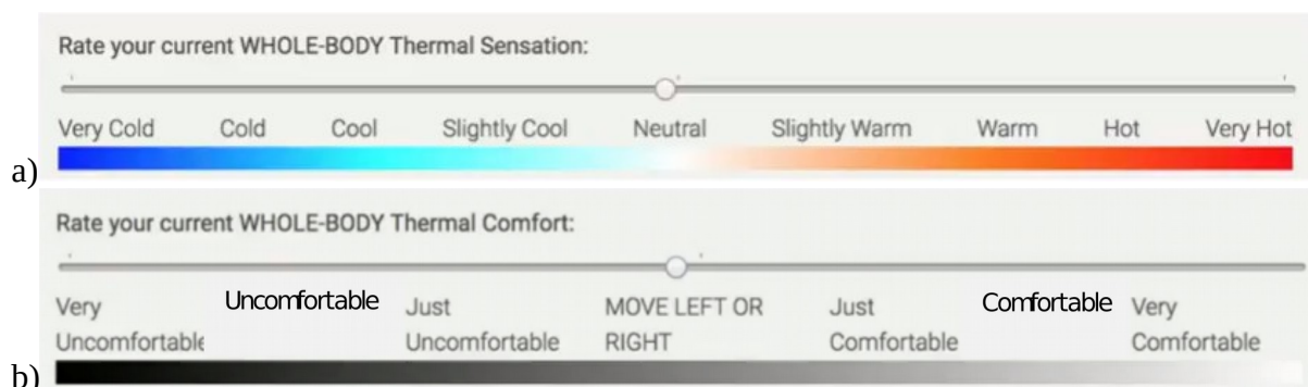
Figure 3. Survey scale a): thermal sensation 9-points scale, b) thermal comfort 7-points scale
