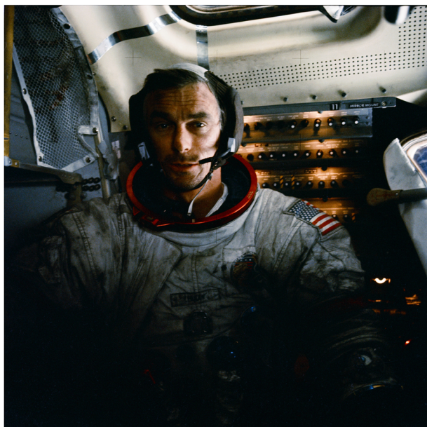
Fig. 3 Lunar dust adherent to spacesuit. Gene Cernan, Apollo 17 commander, is seen with his spacesuit covered in lunar dust following an EVA. Lunar dust can also be seen adhering to the interior of the lunar module 83 . Copyright © NASA Public Domain.
