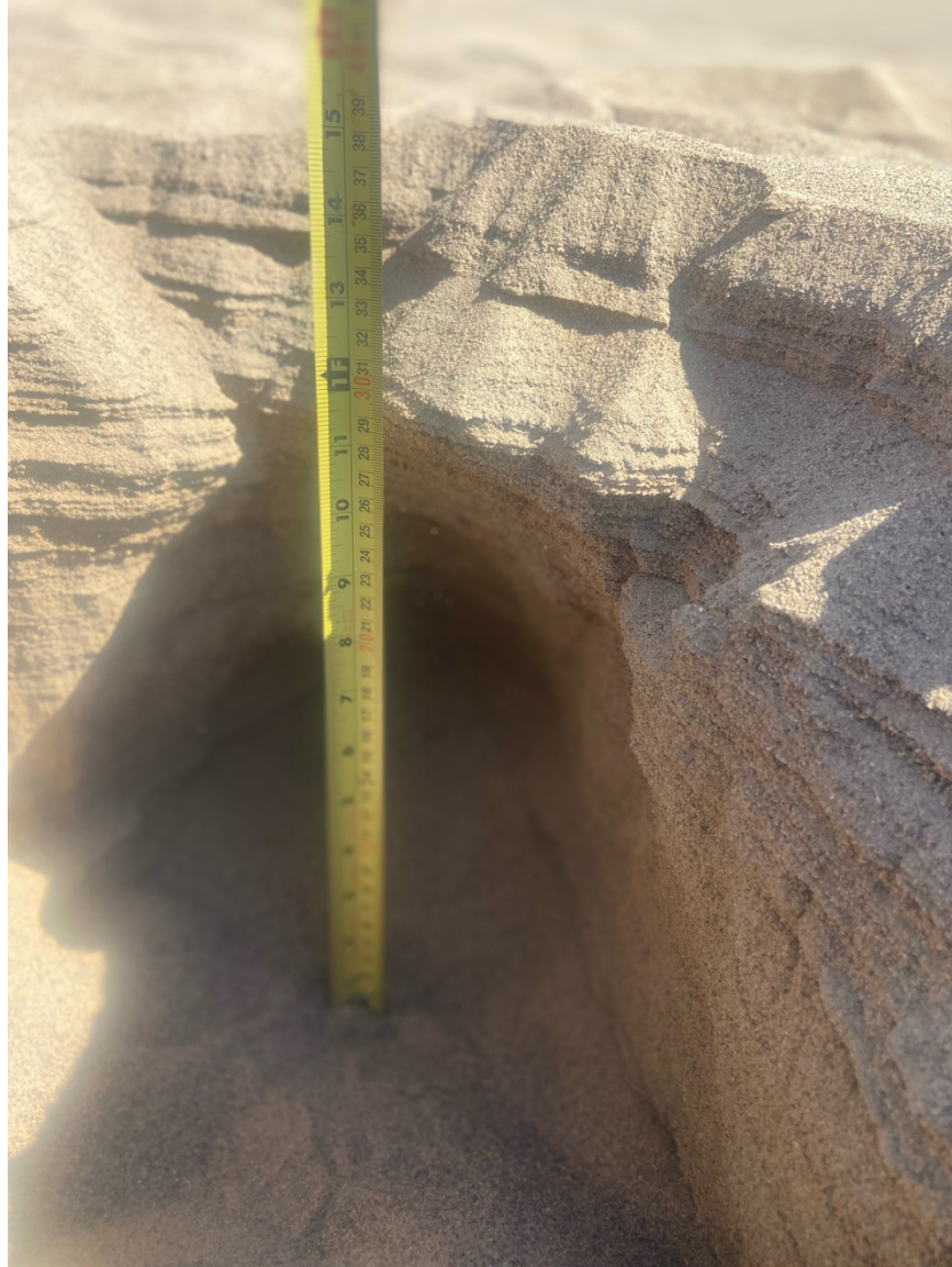
Figure 4.S2 OSL-S Sample location. This image was taken prior to collection of sample OSL-S. This image shows the depth from which the sample was collected, as well as the discernable layers in this portion of the dune. These layers indicate that this portion of the dune has remained stationary since the deposition of these layers.
