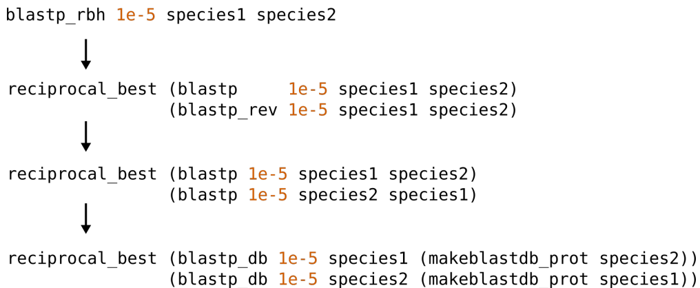
Figure 3.7: Expansion of function calls. Some functions can be easily expressed in terms of other, simpler intermediates. ShortCut expands them during the compilation step. The internal data structure saved (see Figure 3.6) contains the first (top) version, so upon saving it recreates the original code. The compiled file-building rules are based on the last version.
