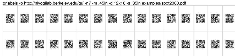
Figure A.3: QR codes suitable for printing on “Tough Spot” freezer-safe stickers. The qrlabels script generates small QR codes with a custom prefix + random UUID. Set the prefix to a database query URL to look up sample information via smartphone.
