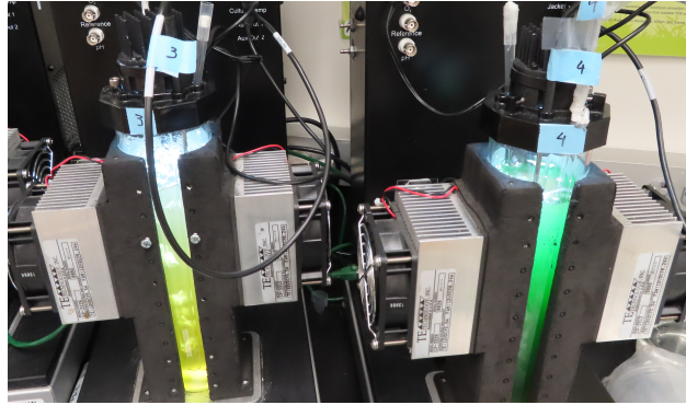
Figure 2.17: PBR culture collapse. Left: collapsed culture. Right: healthy culture.
