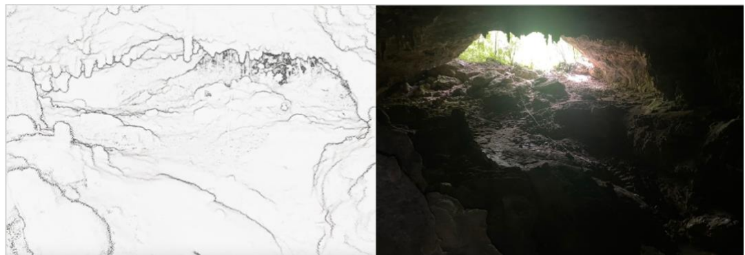
Fig. 2: A comparison between the pointcloud of Las Cuevas entrance and the real world.
