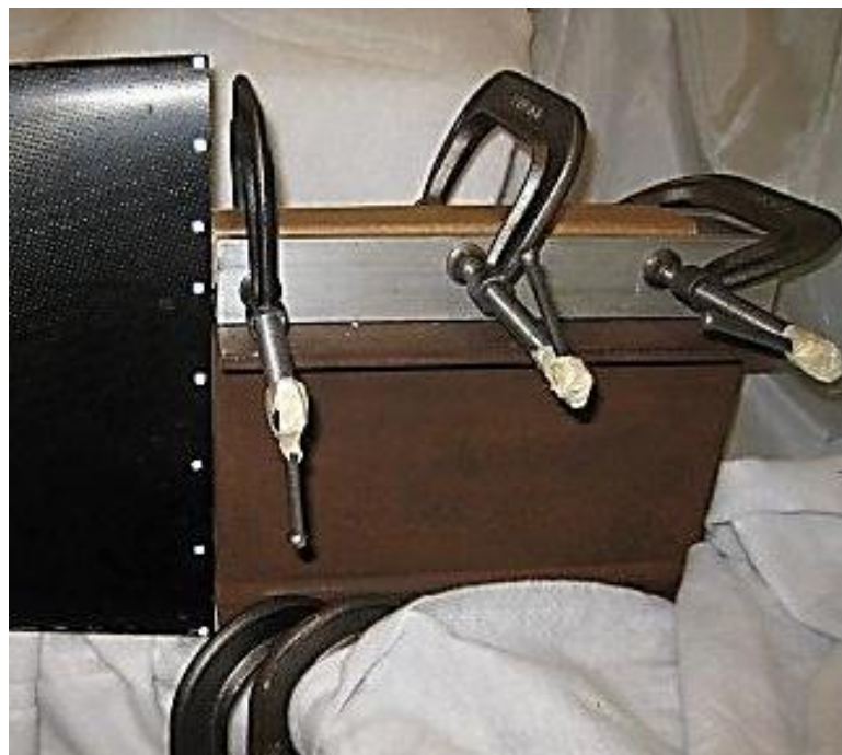
Figure 7-45: Detail of cantilever test fixture.
