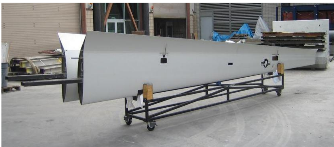
Figure 7-2: Predator UAV wings removed from the rest of the aircraft.
