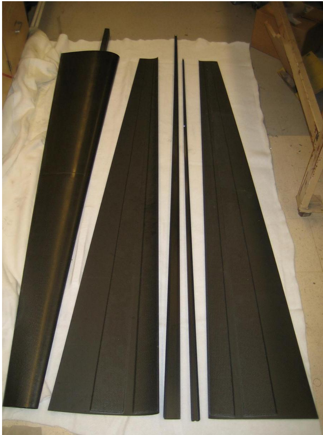
Figure 7-33: An assembled wing (far left), and four component wing pieces (from left-to-right): top skin, main spar, aft spar, bottom skin.
