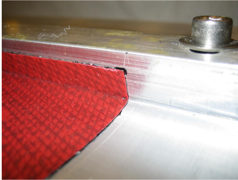
Figure 7-27: Close-up view of bottom wing skin ply formed against the leading-edge joggle tool.
