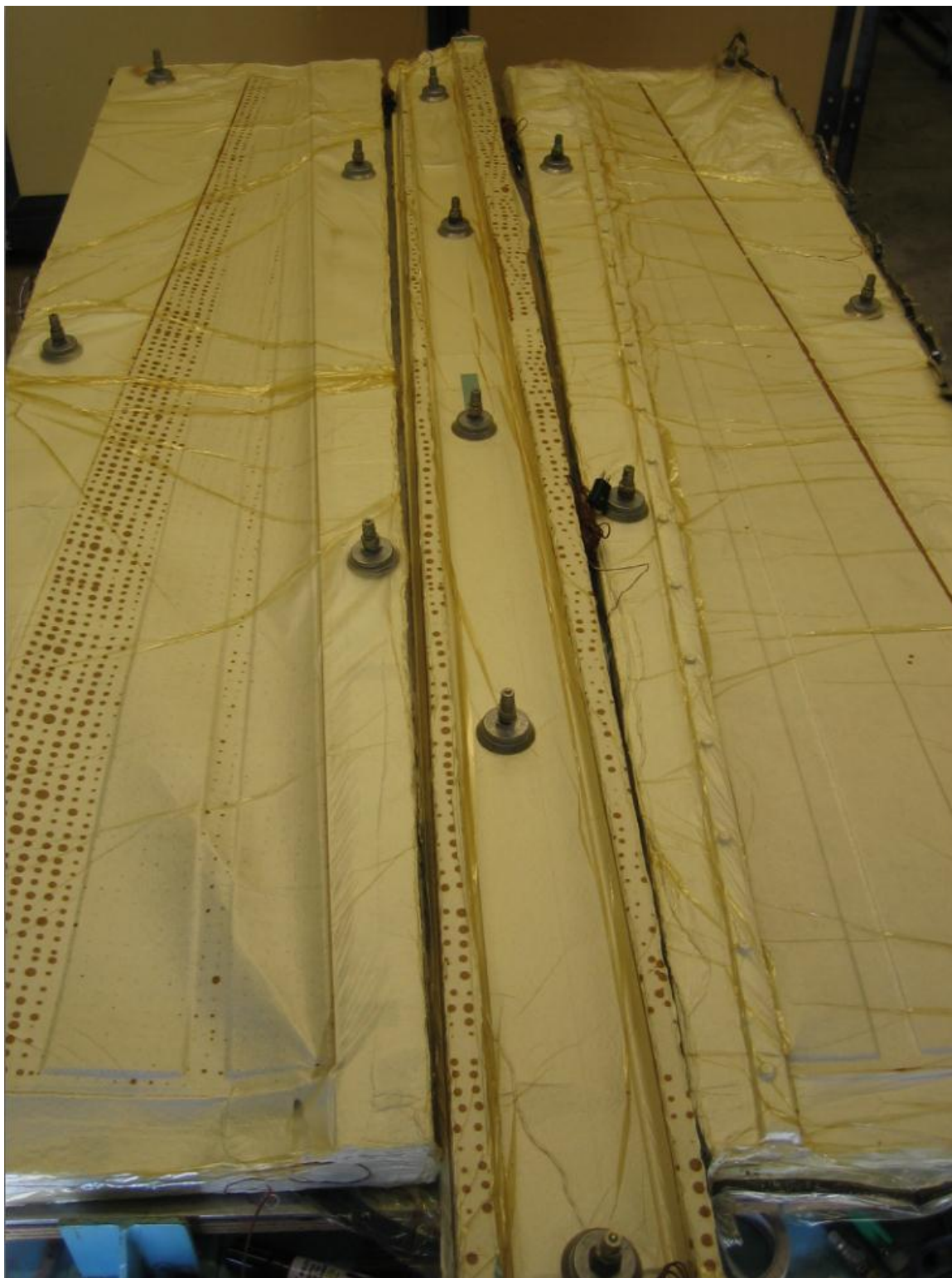
Figure 7-32: Bagged wing components on molds post-cure.
