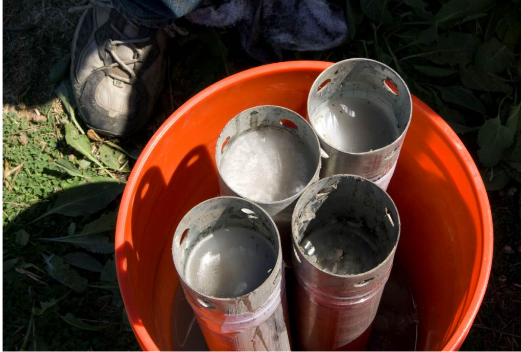
Figure 3.20: Shelby tube samples stored in bucket of water with wax placed on top of specimen.
