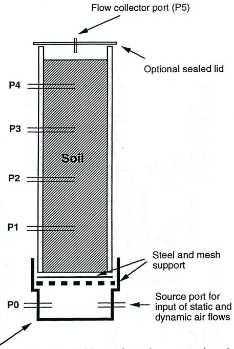
Cap seals to pipe, holding perforated support and mesh
