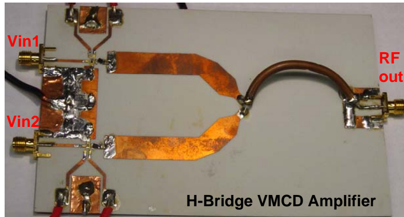
Figure 3.9: The prototype H-bridge class-D power amplifier.
