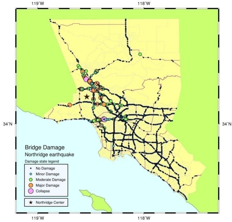
Figure 4.3 Bridge initial damages at Northridge earthquake based on the records.
