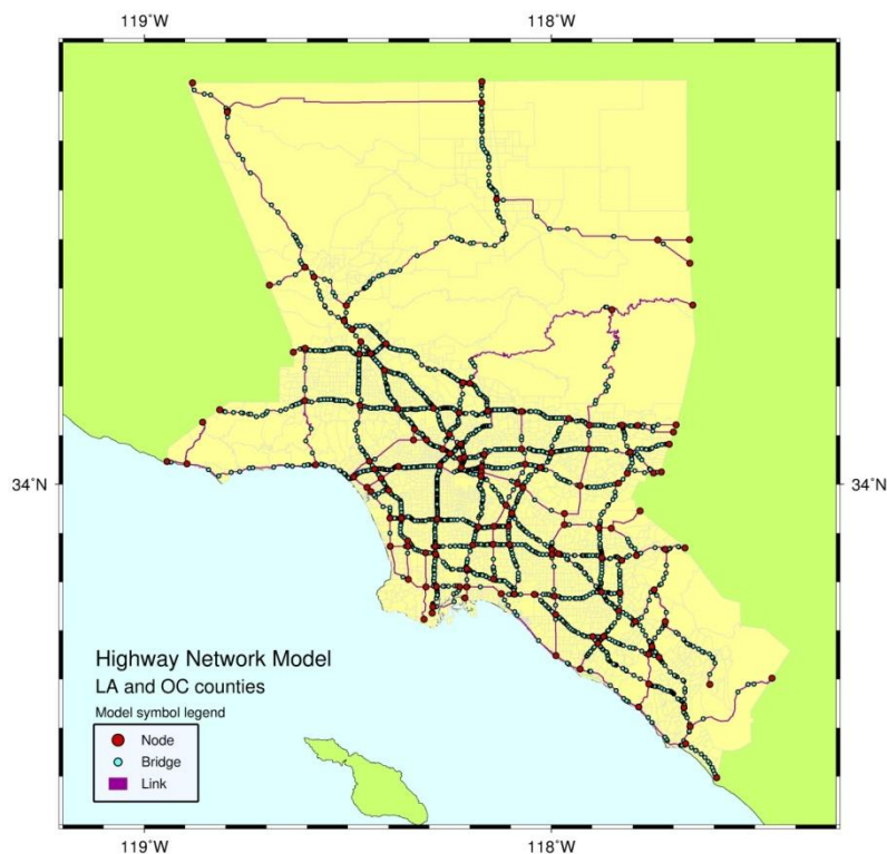
Figure 2.1 Highway transportation network model.
