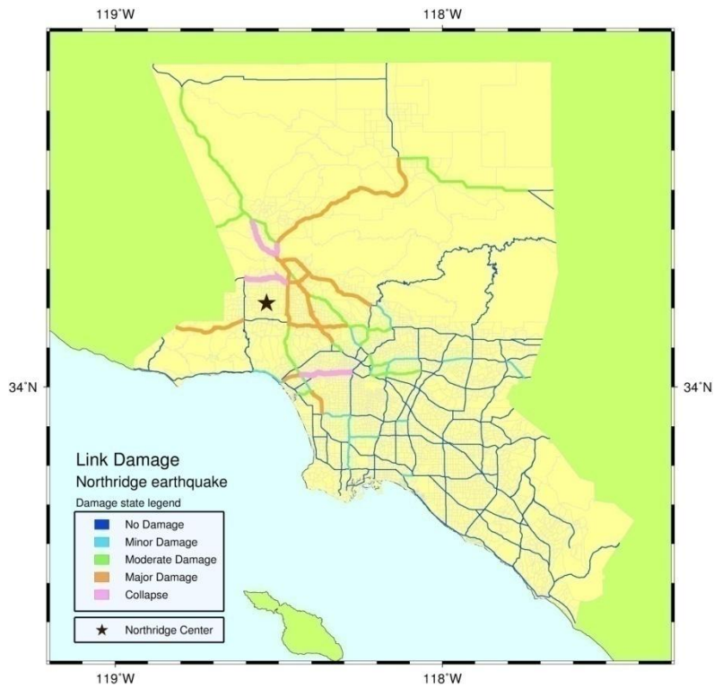
Figure 4.4 Link initial damages at Northridge earthquake based on bridge damages.
