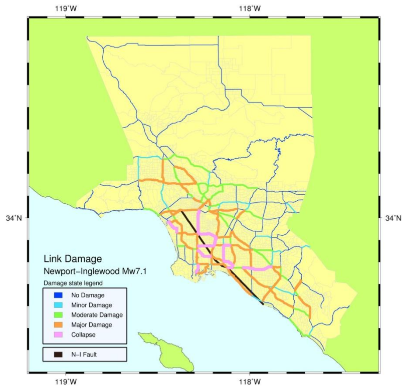
Figure 5.4 Link initial damages by Newport-Inglewood earthquake.
