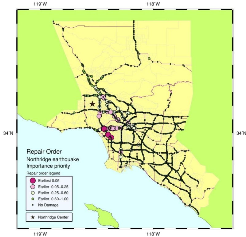
Figure 4.5 Prioritized repair order for Northridge earthquake on Importance.
