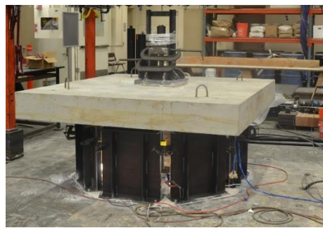
Figure 5– Punching shear specimen (P01) test setup.
