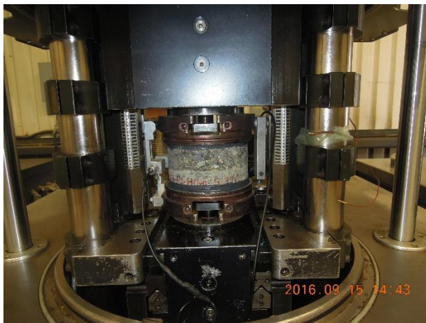
Shear Testing of Composite Specimen. The shear performance of concrete-asphalt interface was tested with the Simple Shear Tester.
