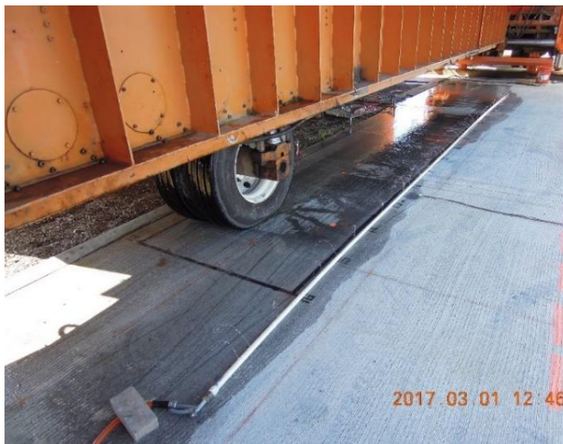
Wet HVS Testing. “Wet” conditions represented a pessimistic field scenario where a pavement drainage system either does not exist or functions very poorly.
