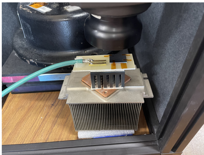
Figure 4.3: Backside imaging sensor setup before the felt is lowered down.
