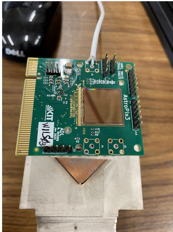
Figure 4.1: Example of sensor placement and bonding for front side image testing.
