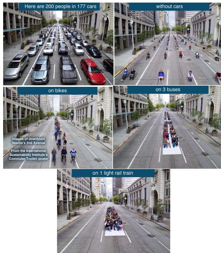
Figure 3.14.: Image sequence from a widely circulated gif produced by the International Sustainability Institute in partnership with the city of Seattle in 2012 as part of their Commuter Toolkit. It shows the space that 200 travelers might occupy in city streets in cars, on bikes, by bus, and on a light rail train. 146
