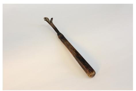
Fig. 2.21: *Kanna* (a small, curved, sharp-edged tool used to make incisions (*hen*) in the tree). Metal, wire, paulownia wood. Image from Japan Lacquer Tapping Technique Preservation Association (Nihon Urushikaki gijutsu hozonkai). https://www.urushikaki-hozon.com/world3/.
