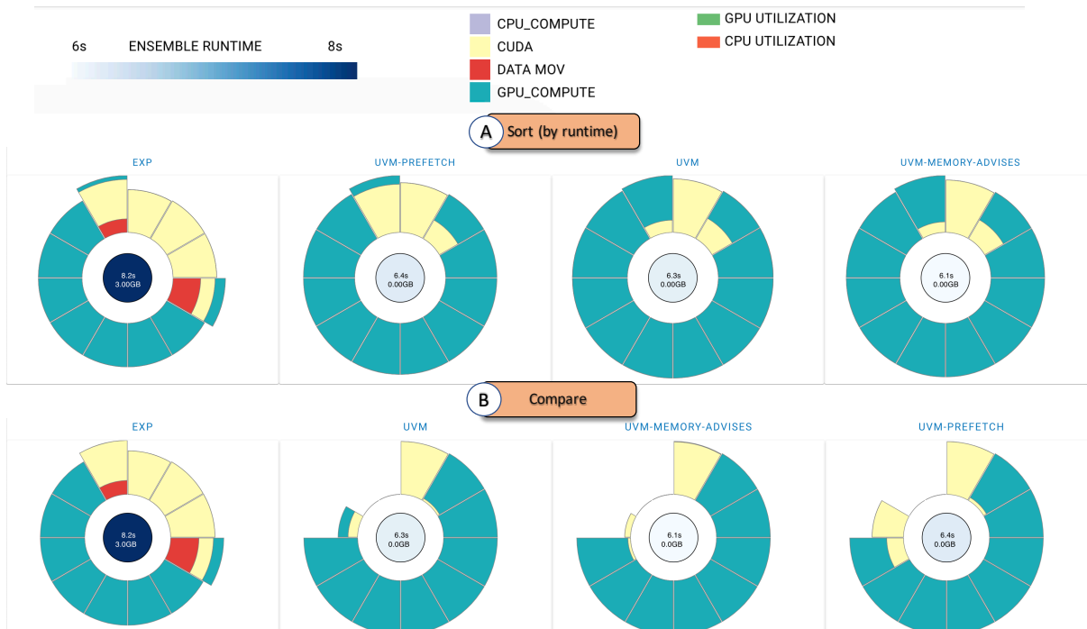
Figure 7.7: GEMM on tall-and-skinny matrices : We leverage the ensemble feature to investigate and compare the time spent across various unified memory management techniques. (A) Sorting the executions by total runtime, from maximum to minimum, highlights that explicit memory transfer is the most time-consuming approach. (B) By comparing the usage of Unified Virtual Memory (UVM) with memory advises and UVM with prefetching, we observe minor differences in the time distribution across CUDA.
