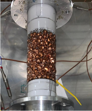
Figure 2.1: Photograph of copper pebble-bed test section.
