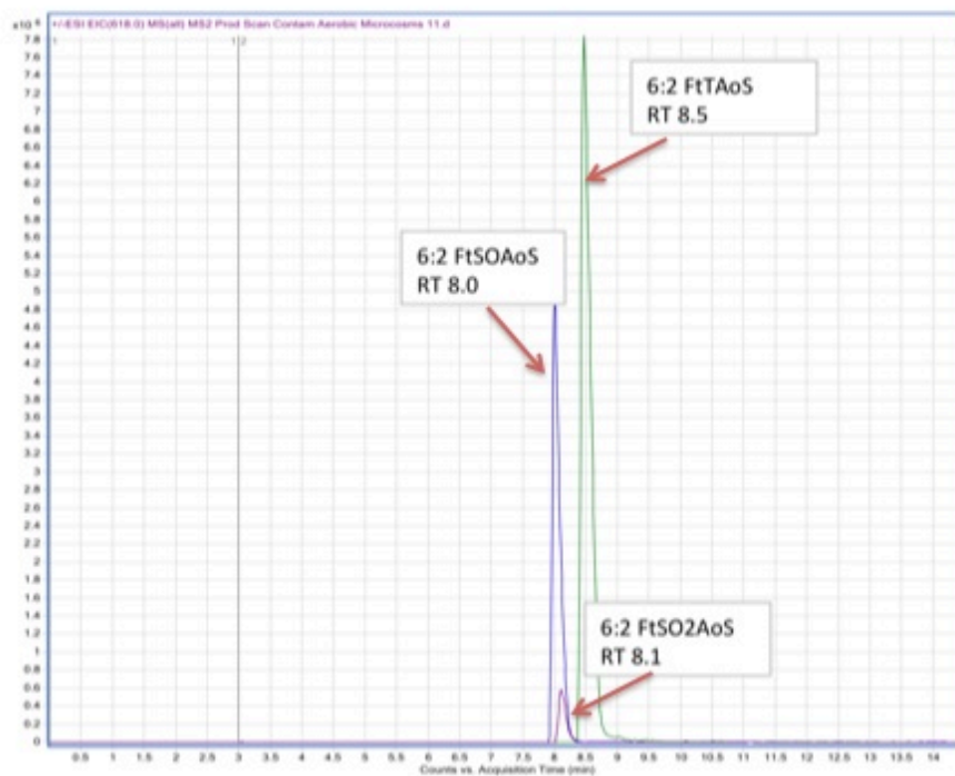
Figure A2.11. Chromatogram of 6:2 FtTAoS (m/z 586), 6:2 FtSOAoS (m/z 602), and 6:2 FtSO 2 AoS (m/z 618) molecular ions in a live microcosm on day 29 of incubation.
