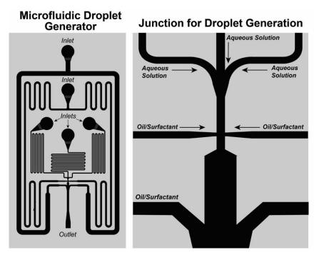
**Figure B21. PicoShell and droplet generator schematic.** Width of channel at the junction for droplet generation is 60µm. Height of channel at junction is 70µm.
