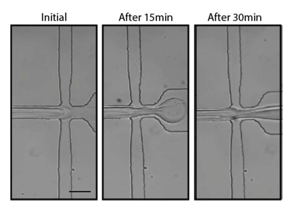
**Figure B19. Disruption of PicoShell generation over time.** Crosslinked material tends to form in the droplet generation junction over time, causing droplet formation to be disrupted. At a pH of 6.5, this usually starts to occur ~15 min after droplet generation is initiated when oversized droplets start to form. After ~30min, no droplets form. The time between initial mixing of reagents and jetting shortens as the pH of the solutions is increased. Scale bar =  $100\mu m$ .
