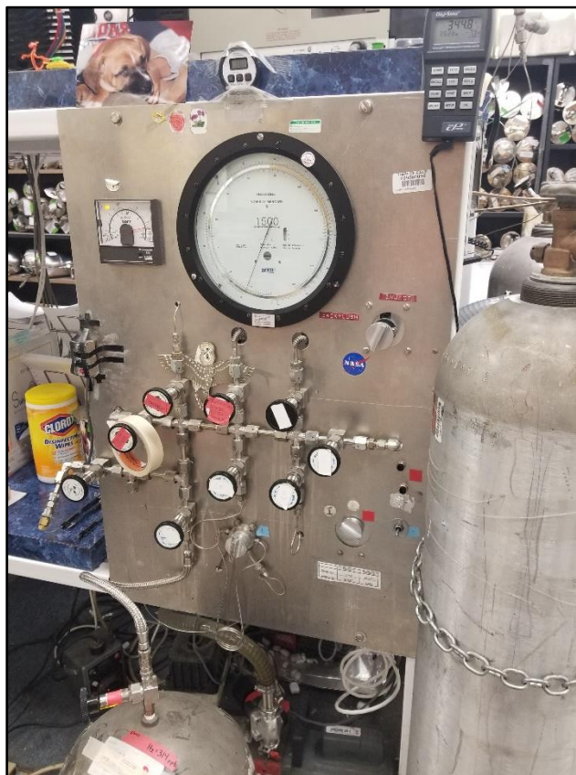
Figure 3.6 Manifold used for analysis of CO and CO 2 in the Rowland-Blake laboratory at the University of California, Irvine. Photograph taken in 2020 by Brenna Biggs.
