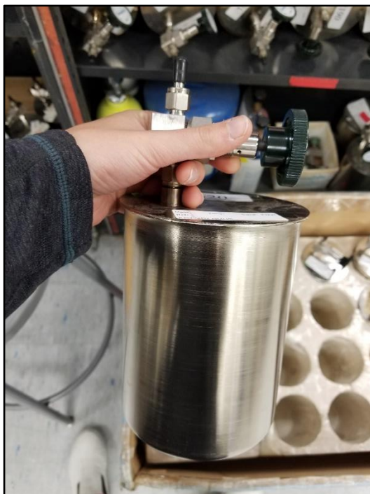
Figure 3.1 A photograph of a 2-liter stainless steel canister used for air sampling. Photograph by Brenna Biggs in 2018.
