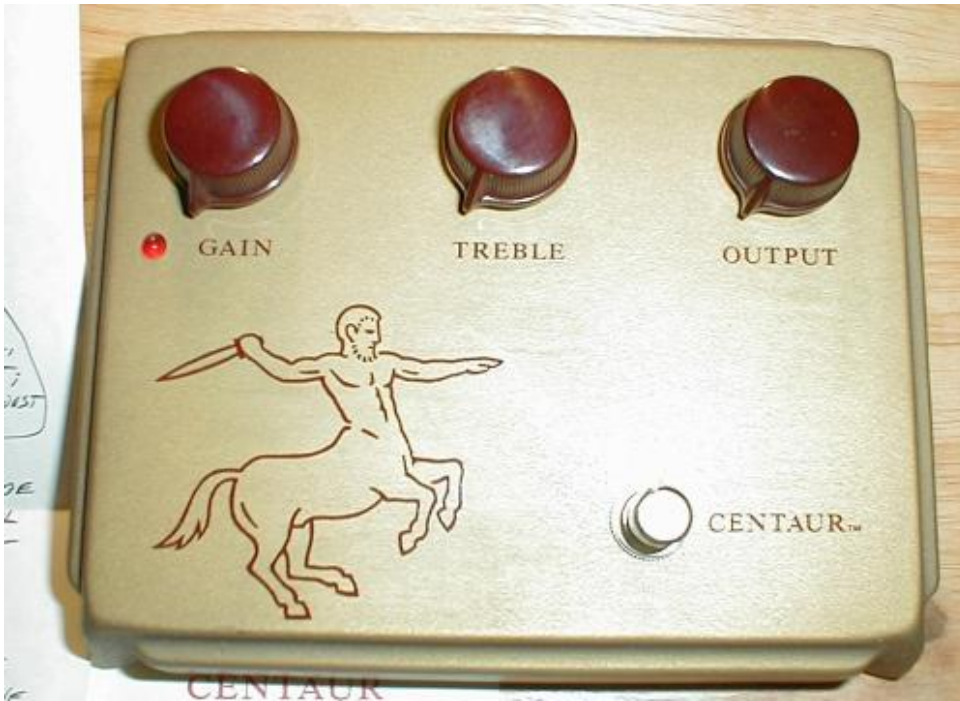
Figure 3.5: The first version of the Klon Centaur overdrive pedal ( http://www.dirtbox.net/news/klon-centaur-is-no-more/ , accessed December 30, 2012)
