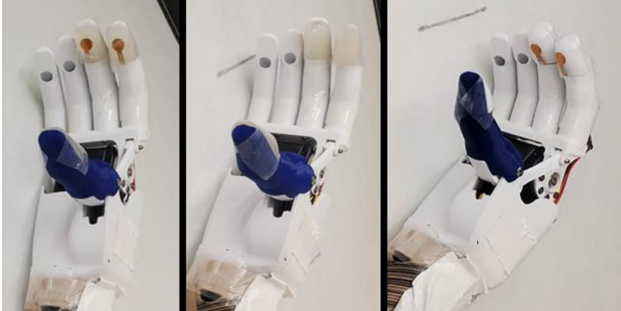
Figure 3.6: The different orientation of the sensors tested during prototype testing. From left to right: sensor above silicone rubber fingertips; sensor below silicone rubber fingertips; sensor above PLA fingertips.
