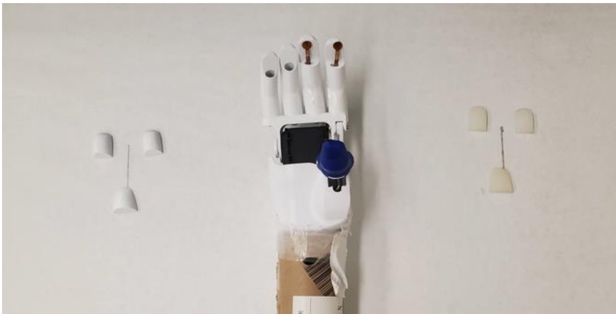
Figure 3.5: Robotic hands with the two types of fingertips: silicone rubber on right, PLA on left.
