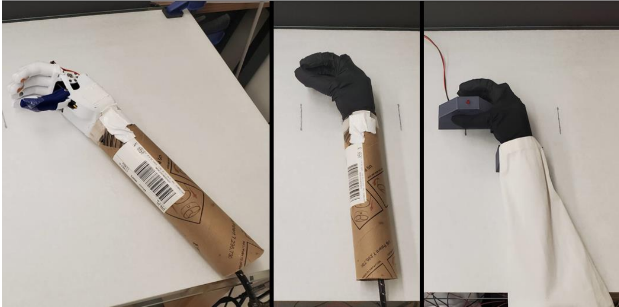
Figure 3.2: Breakdown of robotic hand immersive illusion. From left to right, a cardboard tube is connected to the robotic hand, then a black nitrile glove is worn, and a coat sleeve is attached.
