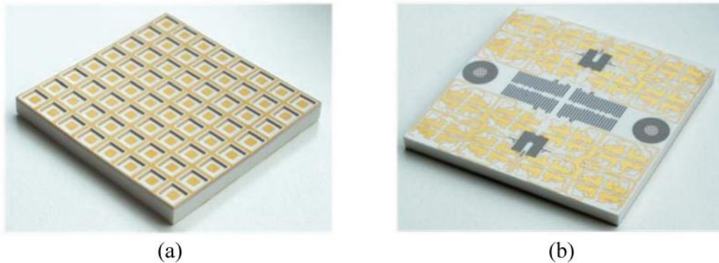
Figure 3.4: Planar Ka-band phased array on LTCC; (a) cavity-backed antenna elements and (b) back-view with RF circuitry [43].
