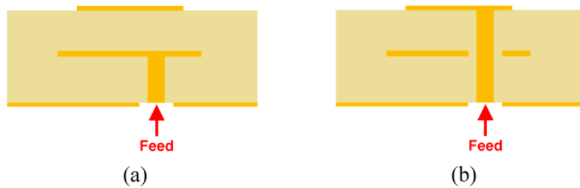
Figure 5.2: Cross-section for (a) wideband and (b) dual-band layered microstrip antennas.
