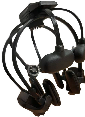
Figure 1.2: EEG equipment. Mobile, dry EEG headsets designed by Cognionics and employed to collect neural data.
