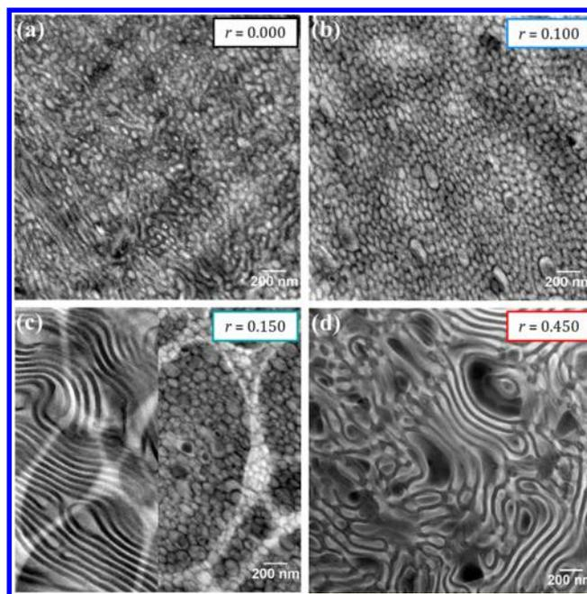
**Figure 2.** STEM micrographs of selected electrolyte concentrations. (a) SEO(52–55)/LiTFSI ( $r = 0.000$ ); (b) SEO(52–55)/LiTFSI ( $r = 0.100$ ); (c) SEO(52–55)/LiTFSI ( $r = 0.150$ ); and (d) SEO(52–55)/LiTFSI ( $r = 0.450$ ). Bright regions indicate PEO-rich phases. The micrograph in (c) is a composite of two separate images taken from difference regions of the sample; the scale bar applies to both images. The support used to hold the sample is visible in (c).
