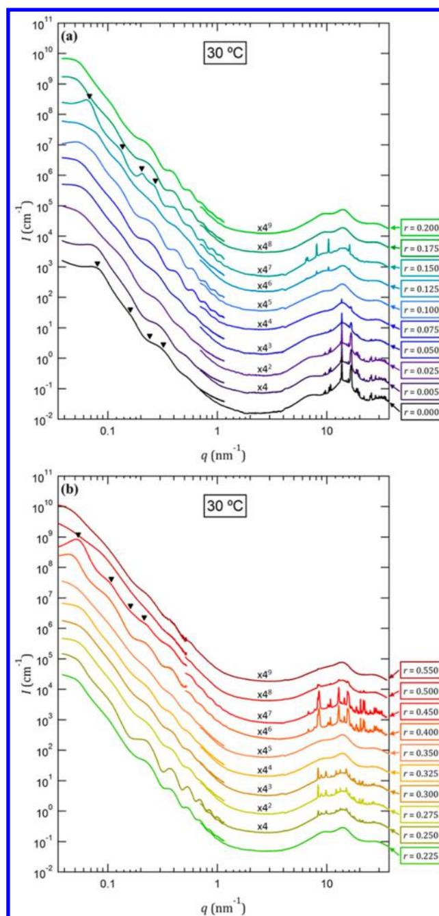
**Figure 1.** Combined SAXS/WAXS profiles for the SEO(52–55)/LiTFSI electrolytes at 30 °C for (a)  $r = 0$ –0.200 and (b)  $r = 0.250$ –0.550. Each salt concentration is indicated by a data tag. Intensities are absolute, but offset by the factors indicated on the plot for clarity. Filled upside-down triangles represent the expected peak positions for a lamellar morphology.
