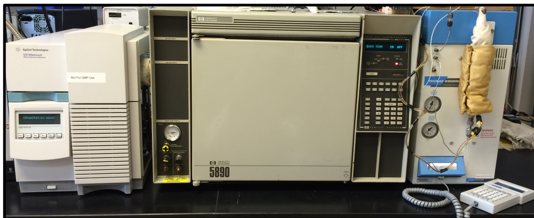
Figure 6.1. Analysis set-up. Left to right: Agilent 5973 mass spectrometer, HP 5890 gas chromatograph, and Tekmar Sample Concentrator.
