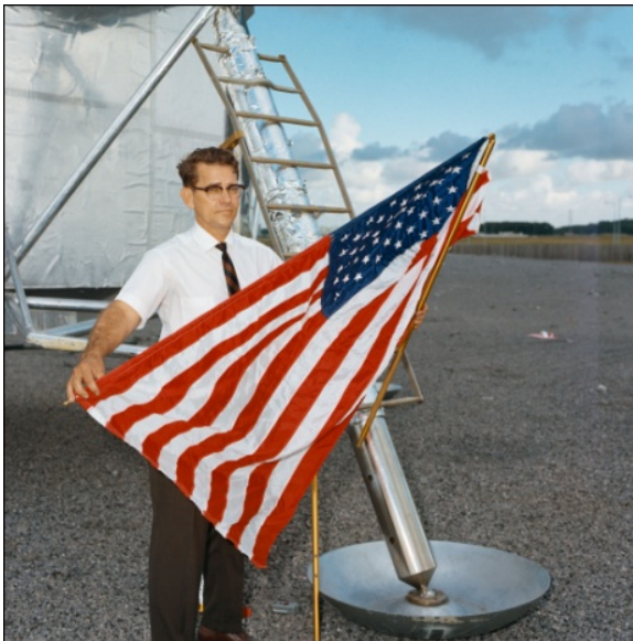
Figures 30–31: After extending the horizontal bar, he lifts the top of the flag up until the latch catches and it stays up on its own (left). He then slides the lower portion of the hoist down to its proper position (right). (NASA JSC Photos S69-38761, S69-38762).
