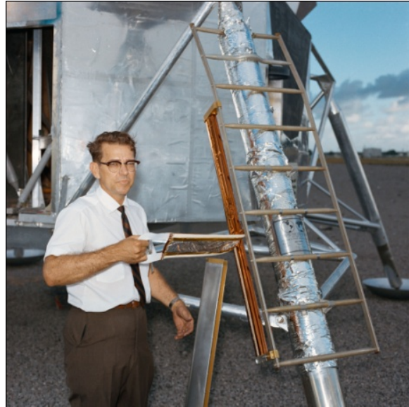
Figures 24–25: A NASA engineer (on Earth) indicates the location where the lunar flag assembly was mounted on the ladder of the lunar module for Apollo 11 and 12. After removing the protective shroud (left), he removes the Velcro strips in order to open the insulation package (right). (NASA JSC Photos S69-38755, S69-38756).
