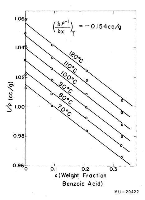
Fig. 28. Reciprocal densities of liquid naphthalene-benzoic acid mixtures. Isothermal plots <u>vs</u> concentration.
