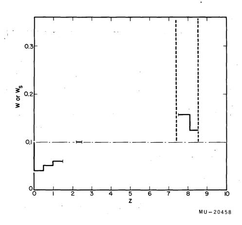
Fig. 70. Experimental concentration profile resulting from a single zone pass of 10%w benzoic acid. Run B-19 (0.15 cm/hr, 10-mm tube pulled down).
