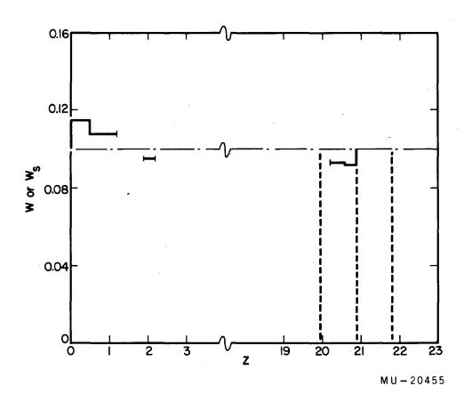
Fig. 67. Experimental concentration profile resulting from a single zone pass of 10%w  $\beta$ -naphthol. Run N-46 (2.7 cm/hr, 20-mm tube pulled down).
