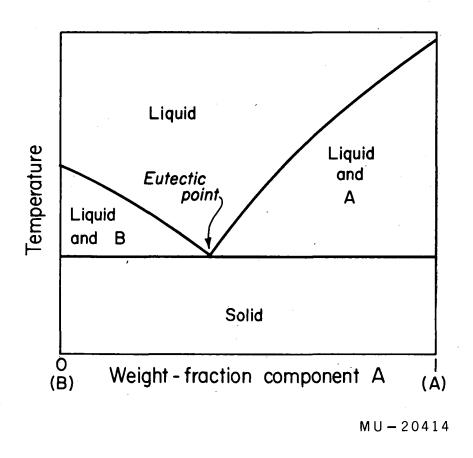
Fig. 7. Solid-liquid phase diagram for a simple eutectic-forming binary mixture (schematic).
