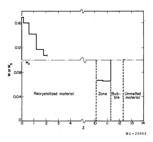
Fig. 65. Experimental concentration (in weight fractions) profile resulting from a single zone pass of 10%w β-naphthol in naphthalene. Run N-44 (0.15 cm/hr zone travel rate, 20-mm glass tube pulled down).
