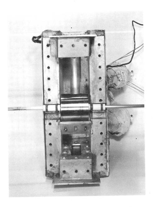
Fig. 18. Top view of the cooled-drum apparatus with the lid removed. Shown are the drum, Teflon and silicone-rubber bearing, doctor blade, temperature-regulator well, and tank outlets (wrapped with heating tape).
