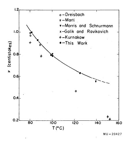
Fig. 33. Comparison of experimentally determined viscosities of naphthalene with literature values.75,78,81-83
