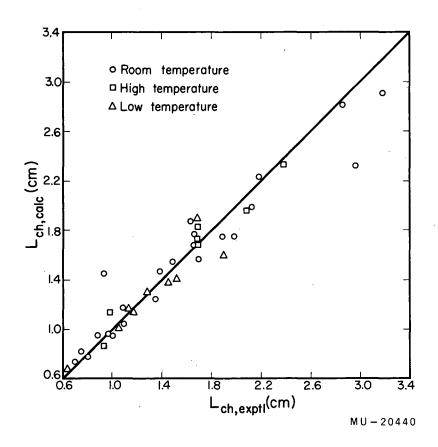
Fig. 46. Comparison of calculated (Eq. 25) with experimental zone locations for vertical zone melting.
