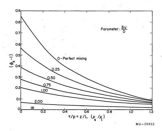
Fig. 64. Concentration profiles resulting from a single zone pass of a material with constant k=1.85, with the bulk of the zone well-mixed.  $(\phi_s-1)$  vs  $\tau/p$ .
