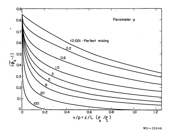
Fig. 58. Average concentrations from 0 to  $\tau$  resulting from a single zone pass of a material with constant k of 1.85, with pure diffusional mass transfer.  $(\phi_s - 1) \underline{vs} \tau/p$ . Calculated from Fig. 57.
