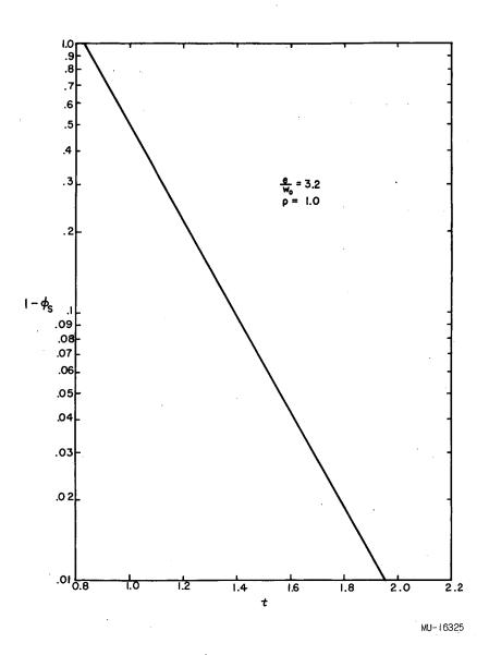
Fig. 54. Exponential portion of a finite-difference solution for pure diffusional mass transfer in zone melting of eutectic formers.  $\ln (1 - \phi_s^-) \underline{vs} \tau \text{ for } \epsilon = 3.2, p = 1.0.$
