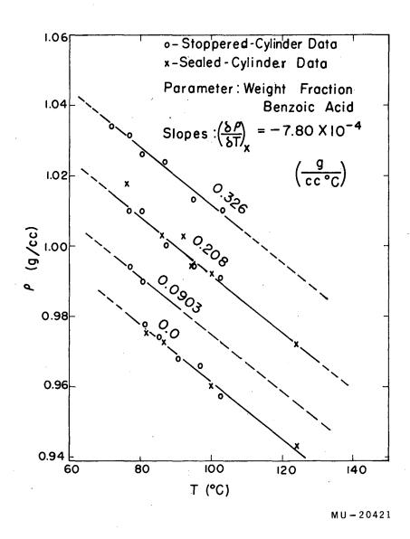
Fig. 27. Densities of liquid naphthalene-benzoic acid mixtures. Constant concentration plots  $\underline{vs}$  temperature.
