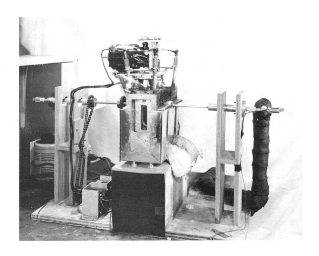
Fig. 15. Photograph of the assembled cooled-drum apparatus.
