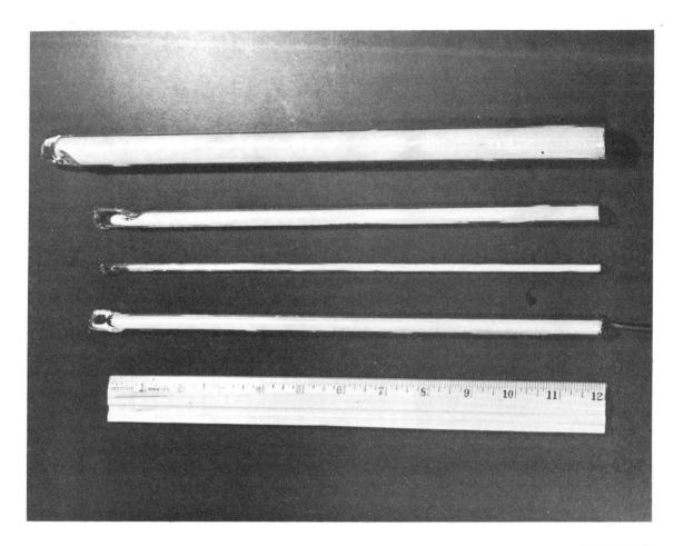
Fig. 13. Photograph of various-sized glass tubes used in zone-melting studies. They have been filled and are ready for use. The scale is graduated in inches.
