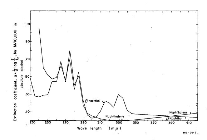
Fig. 37. Literature values of the extinction coefficient plotted  $\underline{vs}$  wavelength for 0.0001 M solutions of naphthalene and of  $\beta$ -naphthol in absolute alcohol. 91
