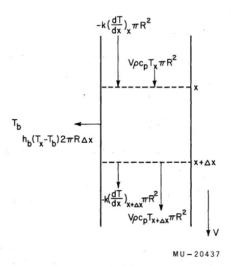
Fig. 43. Differential element of solid, showing heat fluxes.
