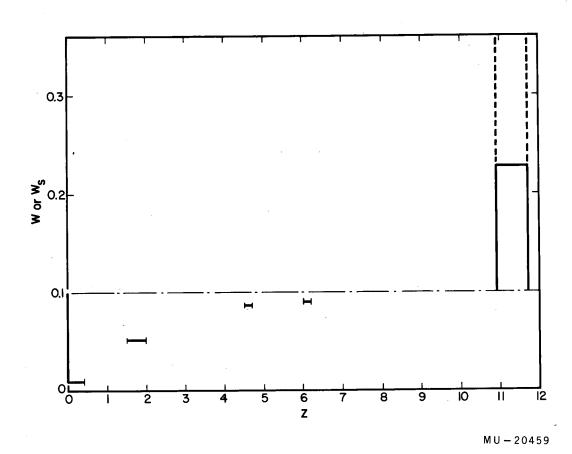
Fig. 71. Experimental concentration profile resulting from a single zone pass of 10%w benzoic acid. Run B-40 (0.45 cm/hr, 20-mm glass tube with a 4-mm axial glass tube in the zone pulled horizontally).
