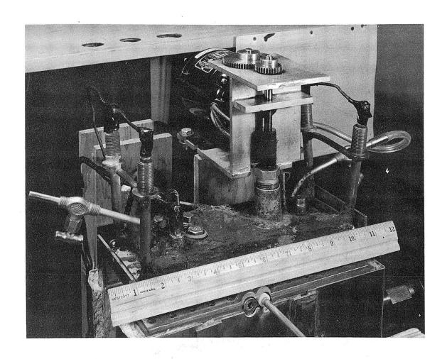
Fig. 16. Top view of the cooled-drum apparatus. Outlets for thermocouple wells, inert gas, heaters, and the stirrer are shown. The scale is graduated in inches.
