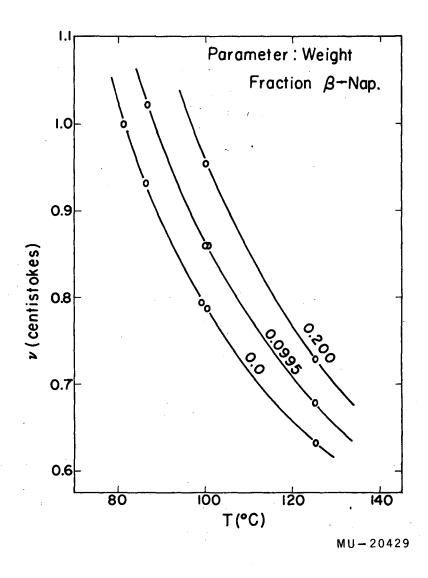
Fig. 35. Constant concentration plots of kinematic viscosity vs temperature for naphthalene-β-naphthol mixtures.
