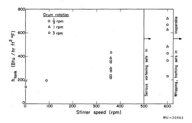
Fig. 75. Observed heat-transfer coefficients between cake surface and molten bath in NaCl-water cooled-drum experiments.
