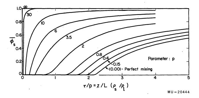
Fig. 56. Average concentrations from 0 to  $\tau$  resulting from a single zone pass of a eutectic-former with  $\epsilon$  = 3.17, with pure diffusional mass transfer.  $\phi_{\rm S} \ \underline{\rm vs} \ \tau/{\rm p}$ .
