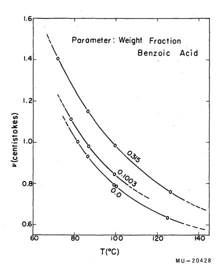
Fig. 34. Kinematic viscosity of naphthalene-benzoic acid mixtures. Constant concentration plots <u>vs</u> temperature.
