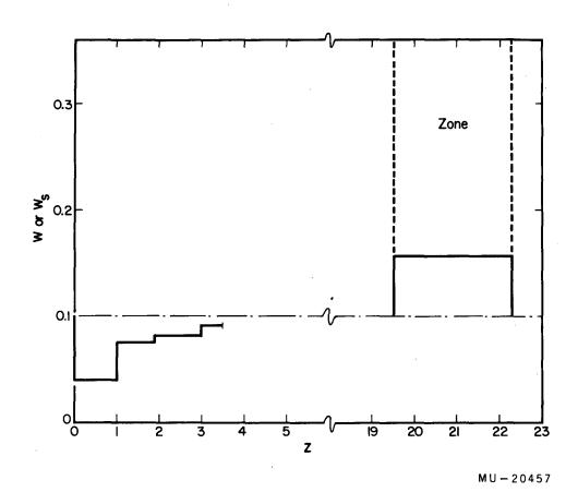
Fig. 69. Experimental concentration profile resulting from a single zone pass of 10%w benzoic acid. Run B-3 (1.35 cm/hr, 10-mm tube pulled up).
