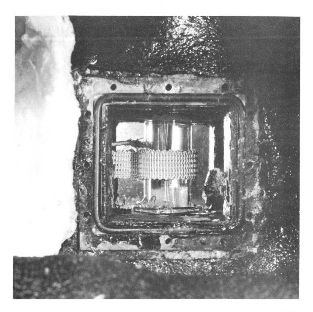
Fig. 14. Close-up of a 0.5-in. heating-tape heater in action (close-up of Fig. 9) on a 20-mm tube with thermocouple leads running axially through it. The freezing interface is visible just below the heating tape.
