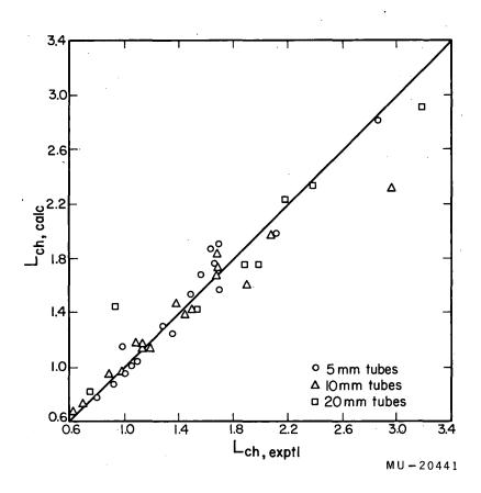
Fig. 47. Comparison of calculated (Eq. 25) with experimental zone locations for vertical zone melting.
