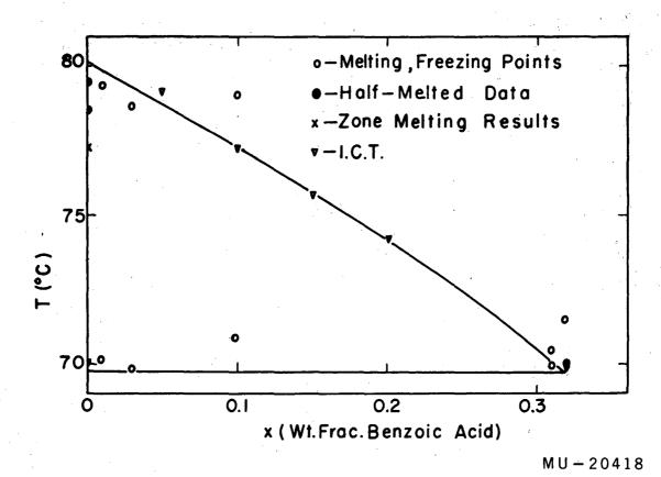
Fig. 23. Naphthalene-rich portion of the solid-liquid phase diagram for the system naphthalene-benzoic acid. Literature values are from reference 58.
