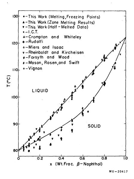
Fig. 22. Solid-liquid phase diagram for the system naphthalene-β-naphthol. Literature values are from references 58 to 65.
