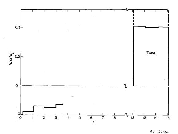
Fig. 68. Experimental concentration profile resulting from a single zone pass of 10%w benzoic acid in naphthalene. Run B-1 (0.15 cm/hr, 10-mm tube pulled up).
