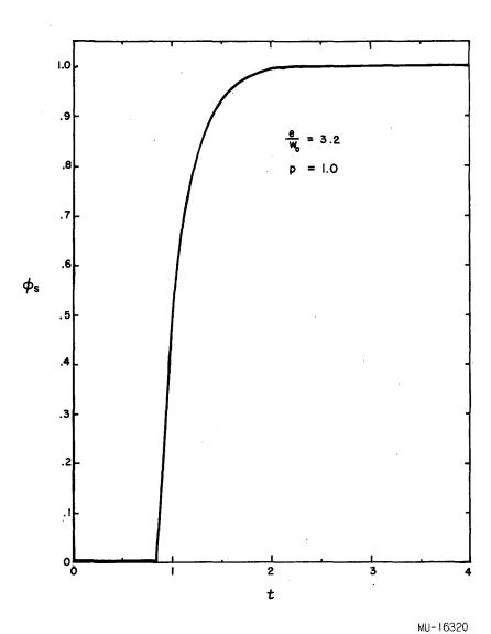
Fig. 53. Sample finite-difference solution for pure diffusional mass transfer in zone melting of eutectic formers.  $\phi_s \underline{vs} \tau \text{ for } \epsilon = 3.2 \text{ and } p = 1.0.$
