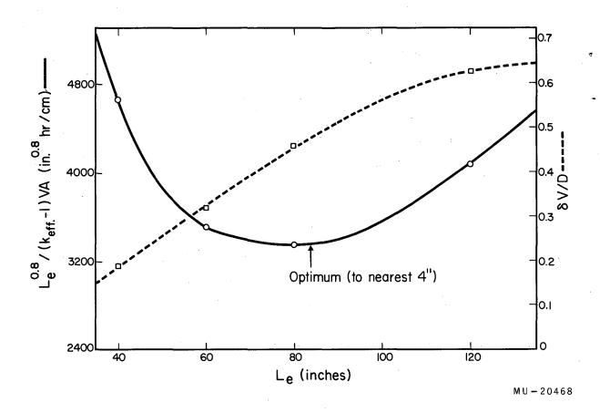
Fig. 80. Relative minimum capital investment necessary for a given production rate of a zone-void refiner.  $(L_e)^{0.8}/(k_{\hbox{\scriptsize eff}}-1) \ \hbox{V A } \underline{\hbox{vs}} \ L_e, \ \hbox{for } \delta=0.05 \ \hbox{cm}.$
