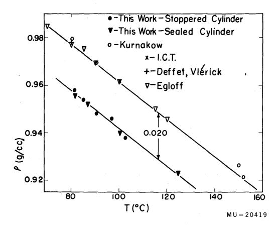
Fig. 25. Comparison of uncorrected experimental values for density of liquid naphthalene with literature values. 58,74,76
