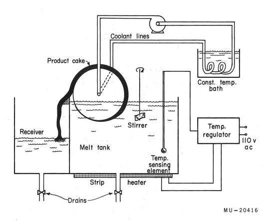
Fig. 19. Schematic diagram of the experimental setup for the cooled-drum apparatus.
