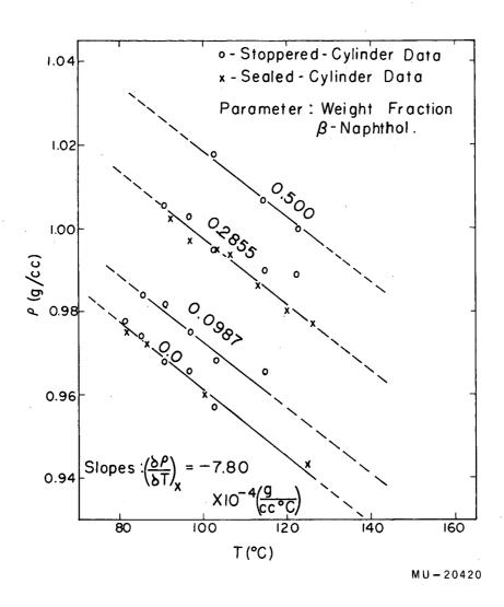
Fig. 26. Densities of liquid naphthalene- $\beta$ -naphthol mixtures. Constant-concentration plots  $\underline{vs}$  temperature.
