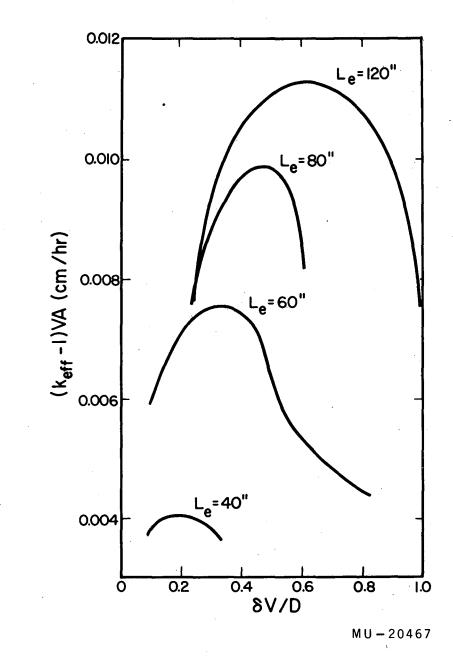
Fig. 79. Relative production rate per zone-void refiner. (k of f = 1) V A vs  $\delta$  V/D, for  $\delta$  = 0.05 cm.
