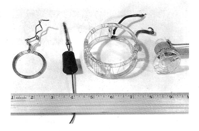
Fig. 12. Photograph of various types of resistance heaters used in zone-melting studies. From left to right are the internal ring heater, probe heater, external ring heater, and heating-tape heater. The scale is graduated in inches.
