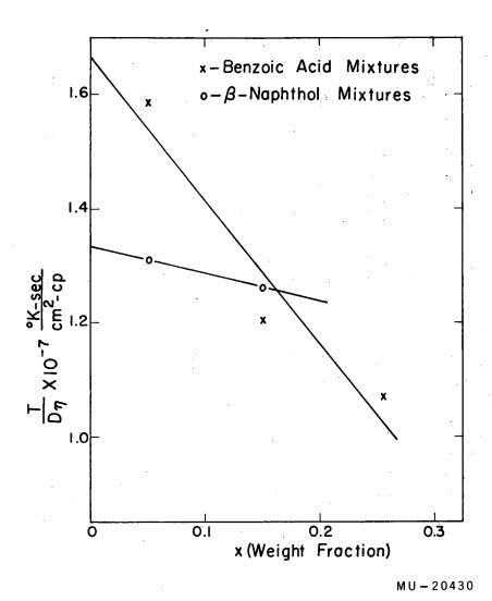
Fig. 36. Values of  $T/D\eta$  vs concentration in weight fraction for naphthalene-benzoic acid mixtures and for naphthalene- $\beta$ -naphthol mixtures.
