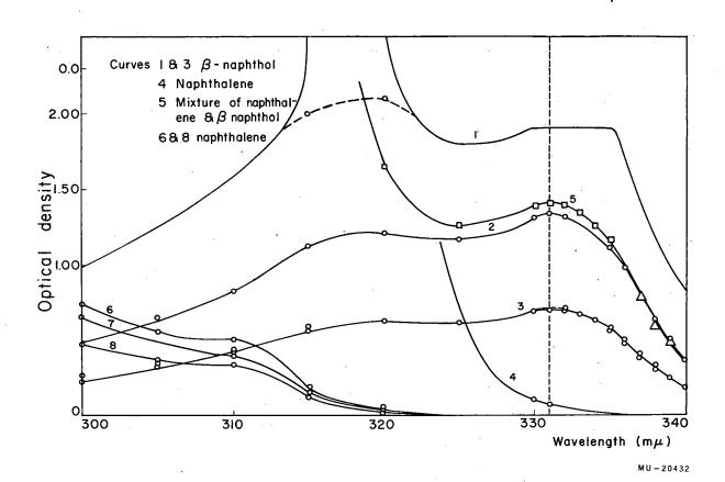
Fig. 38. Optical densities  $\underline{vs}$  wavelength for solutions of naphthalene and  $\beta$ -naphthol in absolute alcohol. Curves are for 25-ml alcoholic solutions of
