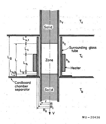
Fig. 42. Diagram showing various thermal parameters in zone-melting apparatus.
