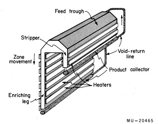
Fig. 77. Diagram of proposed zone-void refiner.
