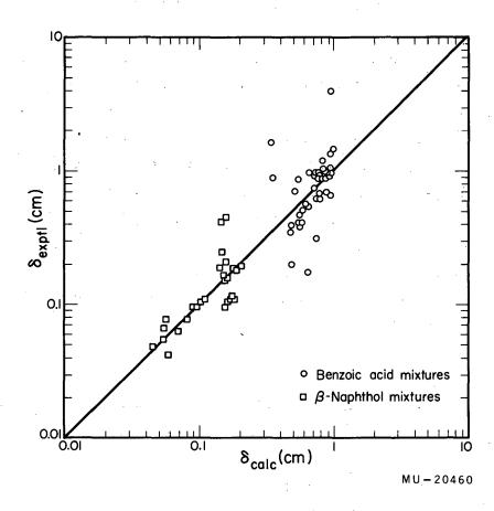
Fig. 72. Comparison of experimental with calculated boundary-layer thicknesses [Eq. (83)] for zone melting runs, with the tube pulled down and with no axial tubes or rods.
