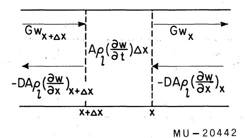
Fig. 49. Differential element of zone showing material fluxes in pure diffusional mass transfer.
