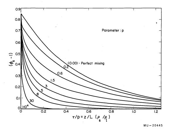
Fig. 57. Concentration profiles resulting from a single zone pass of a material with constant k of 1.85, with pure diffusional mass transfer. ( $\phi_s$  - 1) vs  $\tau/p$ . Calculated from Eq. (64).
