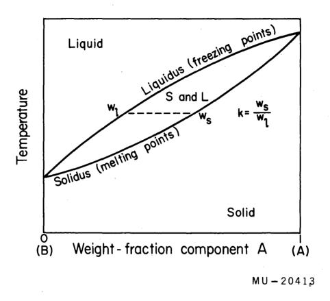
Fig. 6. Solid-liquid phase diagram for a completely isomorphous binary mixture (schematic).
