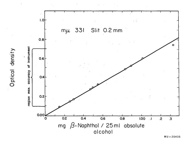
Fig. 41. Standard curve for the spectrophotometric analyses of mixtures of  $\beta\text{-naphthol}$  in naphthalene. Optical density  $\underline{vs}$  mg  $\beta\text{-naphthol}$  per 25 ml of alcoholic solution.
