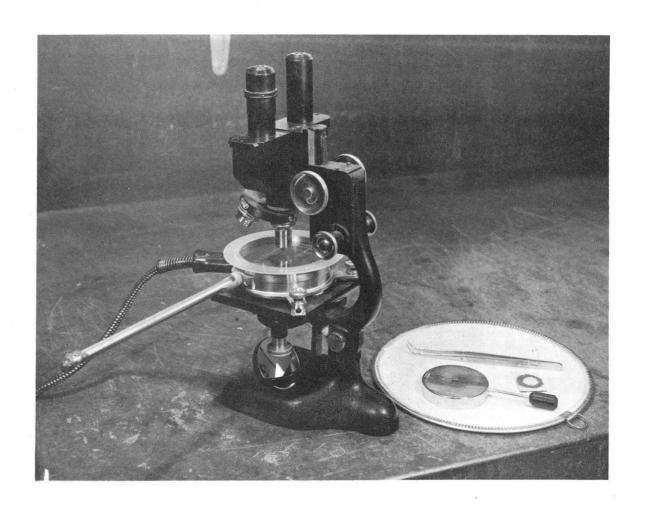
Fig. 20. Photograph of the micro-hot-stage and accessories used for melting-point determinations.
