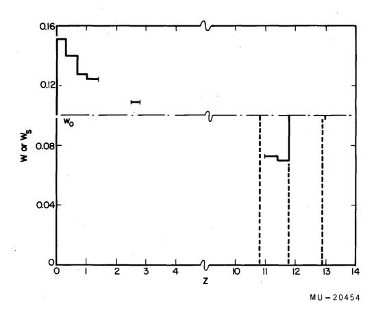
Fig. 66. Experimental concentration (in weight fraction) profile resulting from a single zone pass of 10%w  $\beta\text{-naphthol}$  in naphthalene. Run N-45 (0.45 cm/hr zone travel rate, 20-mm glass tube pulled down).
