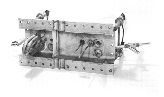
Fig. 17. Bottom view of the lid to the cooled-drum apparatus. Shown are the thermocouple wells, heater for receiving chamber, Teflon chamber-separator, and stirrer (paddle edgewise to the camera).
