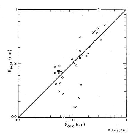
Fig. 73. Comparison of experimental with calculated boundarylayer thicknesses [Eq. (84)] for zone melting runs other than when the tube was pulled down with no axial tubes or rods in it.
