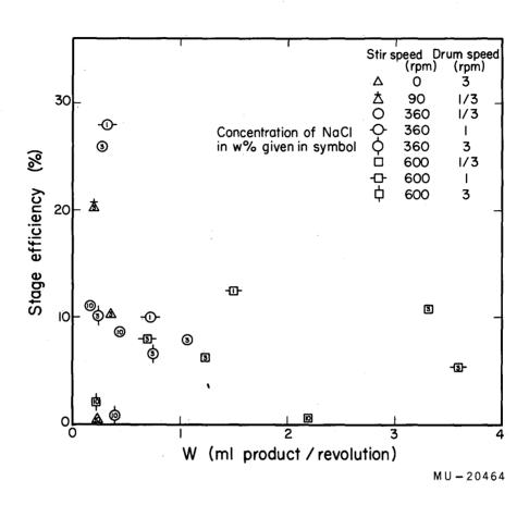
Fig. 76. Stage efficiencies in cooled-drum runs with NaCl-water.
