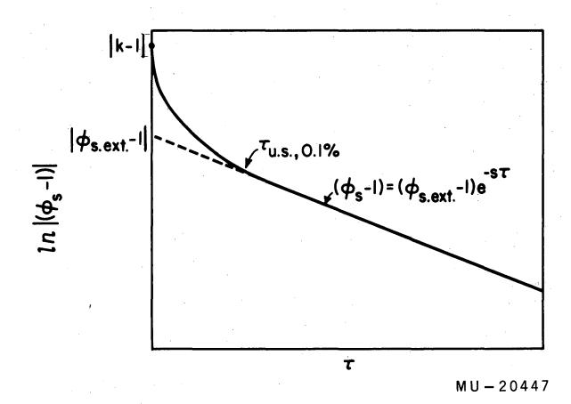
Fig. 59. Schematic sketch of a concentration profile for a single zone pass of a material with constant distribution coefficient, with pure diffusional mass transfer, showing the parameters characterizing the curve.  $\ln |\phi_s - 1| \underline{vs} \tau.$
