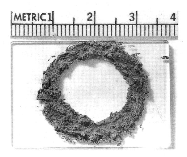
Fig. 21. Close-up of a microscope slide prepared for a melting-point determination. The black material in a circle is Thermon, which seals the cover glass to the slide. The scale is graduated in centimeters.
