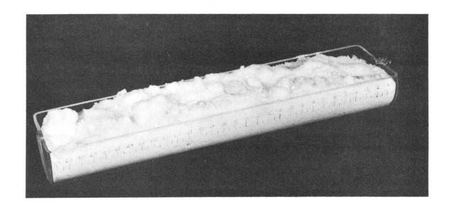
Fig. 11. Photograph of an early open-top boat used for zone-melting studies. The white material was used to make the boat photograph better.
