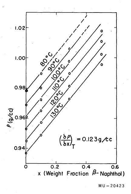
Fig. 29. Densities of liquid naphthalene- $\beta$ -naphthol mixtures Isothermal plots  $\underline{vs}$  concentration.
