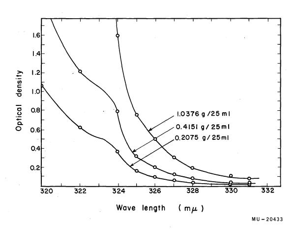
Fig. 39. Optical density  $\underline{vs}$  wavelength for solutions of naphthalene in alcohol.
