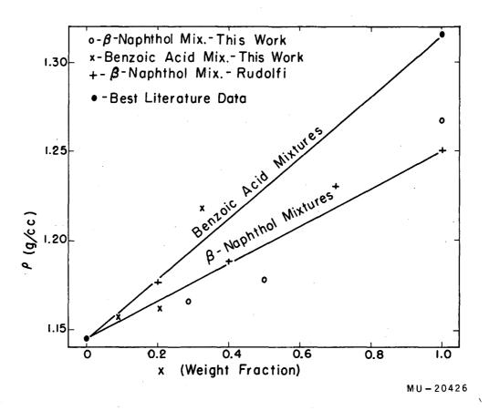
Fig. 32. Solid densities of mixtures of naphthalenebenzoic acid and of naphthalene-β-naphthol plotted vs weight fraction.
