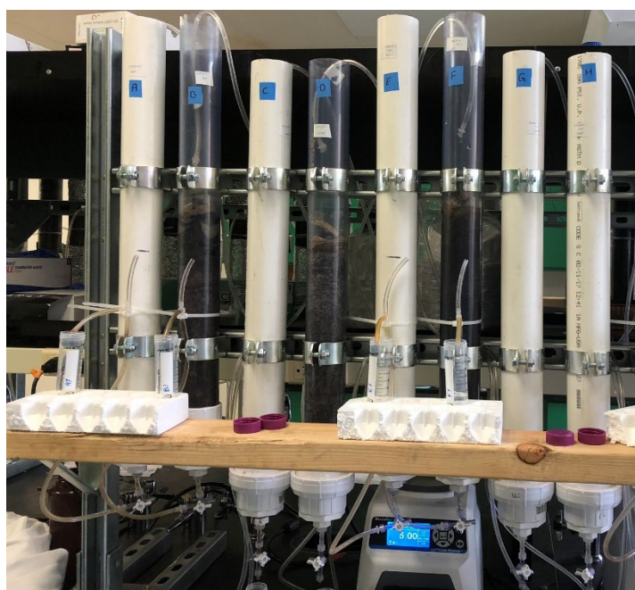
Figure 4-1. Biofilter setup featuring compost and compost + iron with and without a submerged layer.
