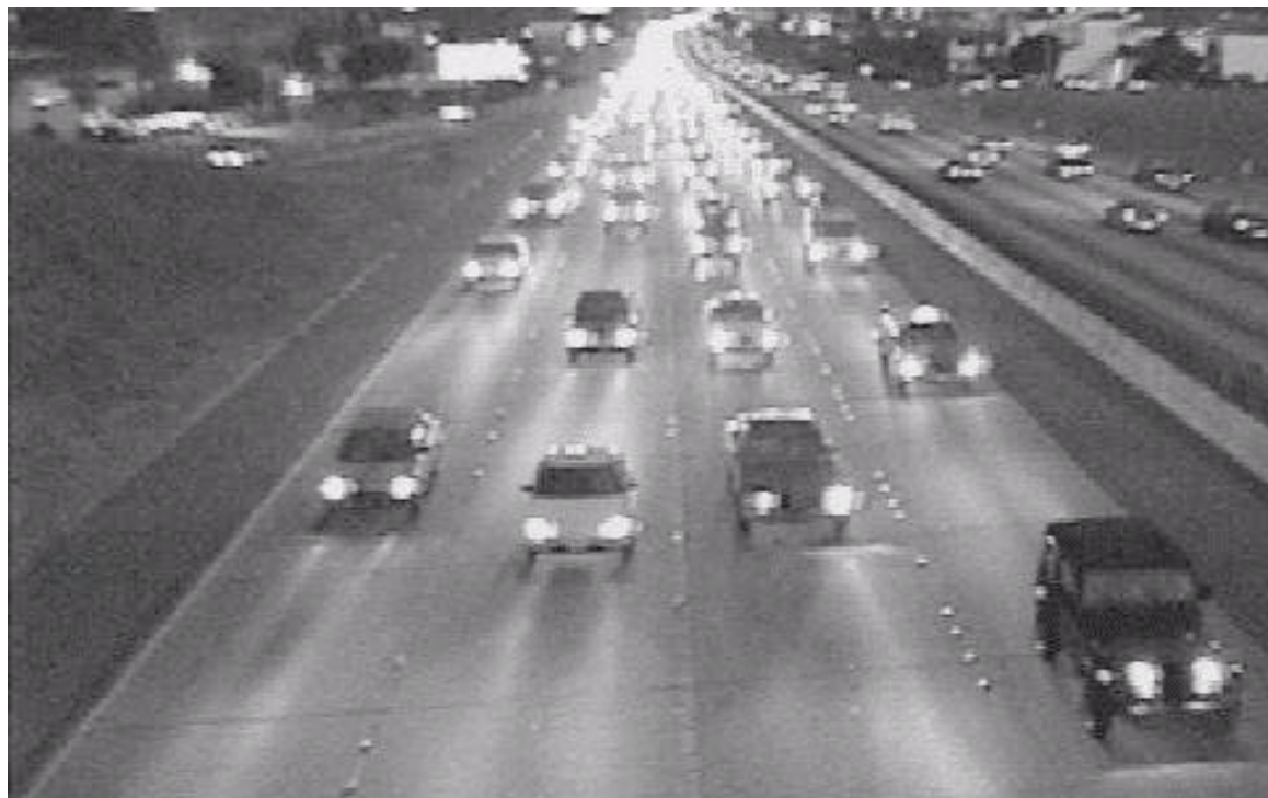
Figure 19. Digitized Video Image of Night Highway Traffic, Burle TC9388-1 Camera, Auto-shutter mode.
