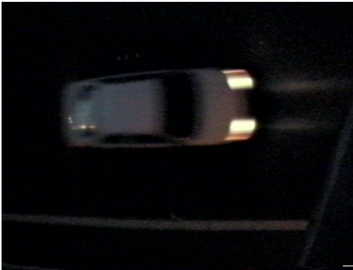
Figure 9. Image Blur Due to Slow Shutter Speed Under Low-Light Conditions.
