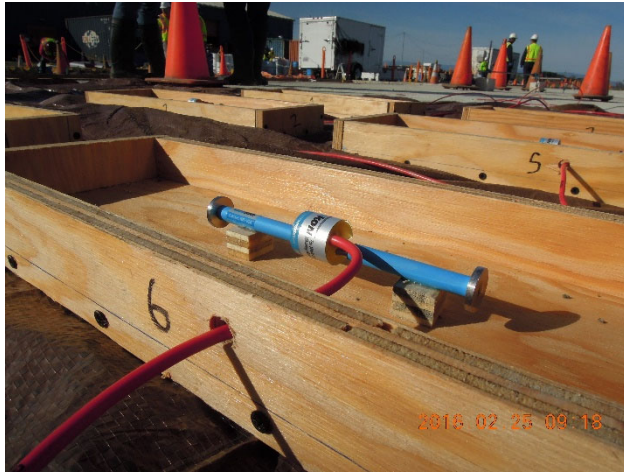
VWSG inside the mold before placing concrete
