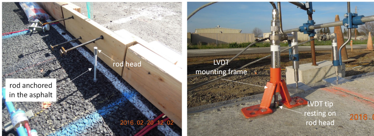
Figure 2.9: Interface opening measuring device (IOMD). (Note: left side shows before concrete placement, right side after concrete placement.)
