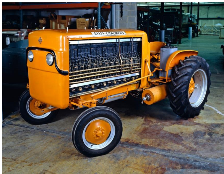
Figure 2-5: Allis-Chalmers' 15 kW fuel cell tractor [49].
