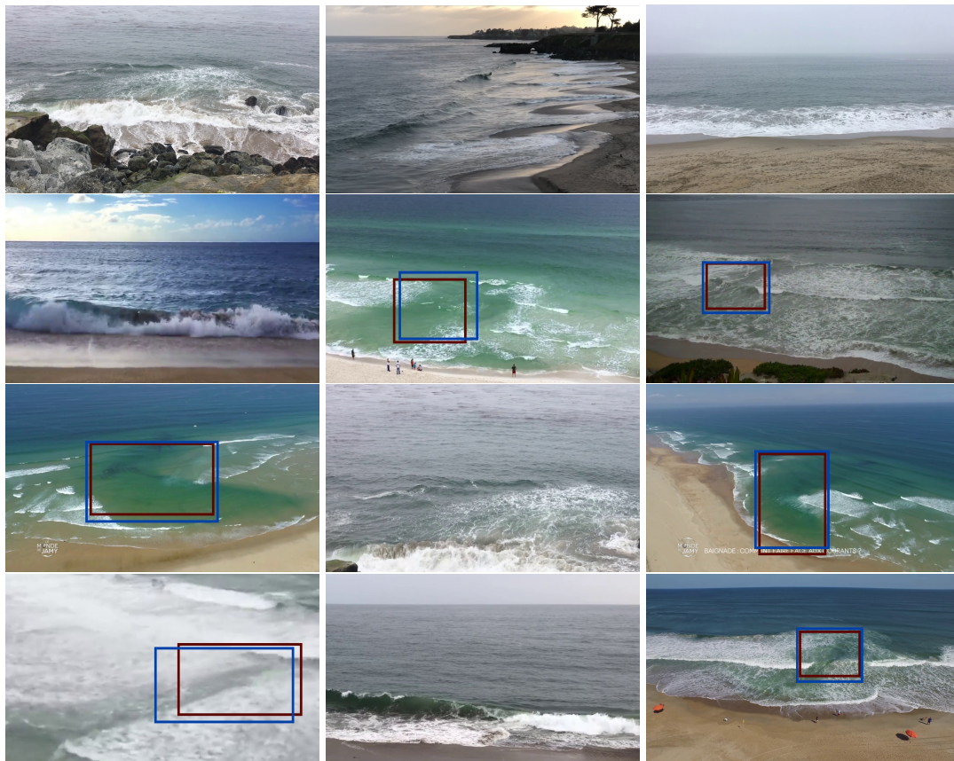
Figure 3.8: Detections: Rip current detections on some of the frames from the test data set. Red bounding boxes show the correctly detected rip currents. Blue bounding boxes show the ground truth. Frames without bounding boxes do not contain any rip currents.
