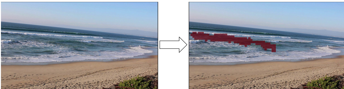
Figure 4.1: Rip currents are deadly but remain invisible to many: We propose a feature detection method, RipViz, to make these invisible rip currents visible. RipViz highlights locations of rip currents as a red region. This region is determined by finding seed points that produce pathline sequences deviating from normal ocean flow. Non-experts and experts alike can use RipViz to visualize rip currents.
