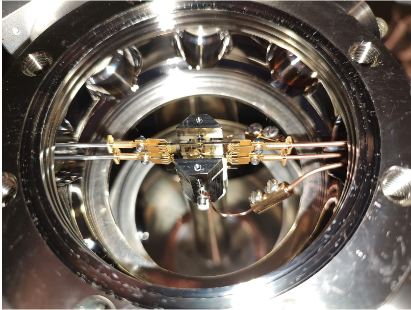
Figure A.1: The new “wheel trap” and electrical connections.
