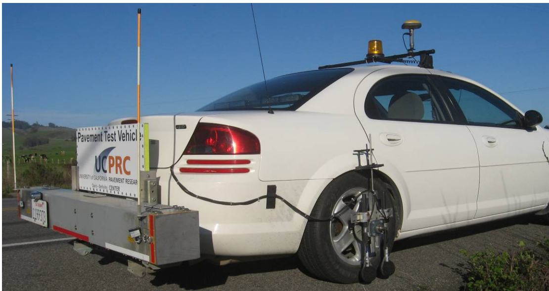
Figure 2: Instrumented vehicle and microphone setup for measuring tire/pavement noise.
