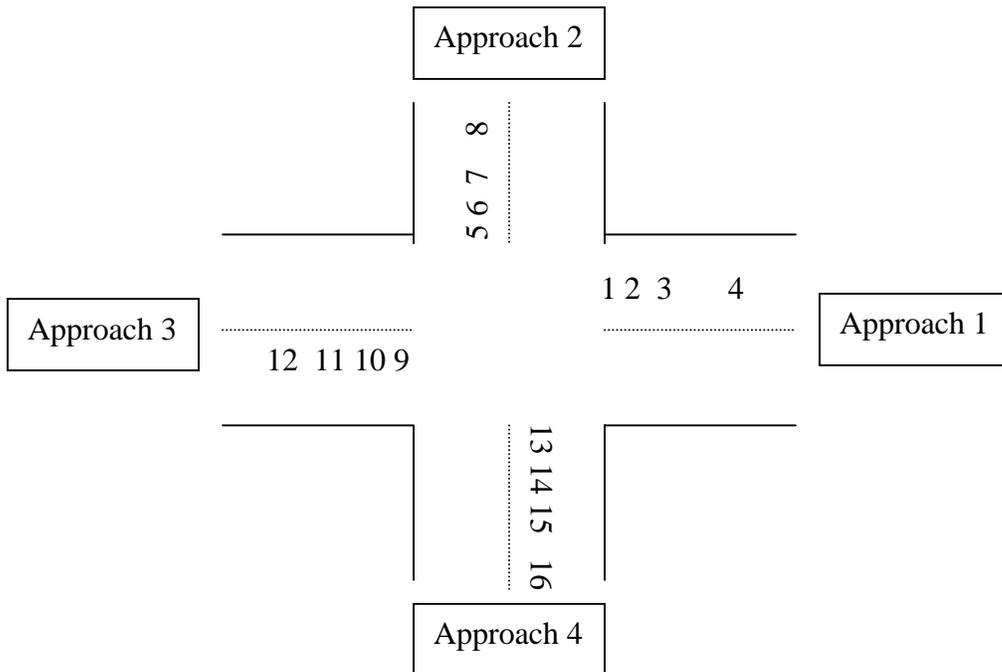
Figure 2 Detector numbering based on NEMA phases
