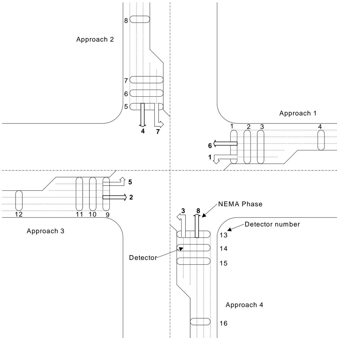
Figure 1. Typical Intersection Layout with NEMA phases
