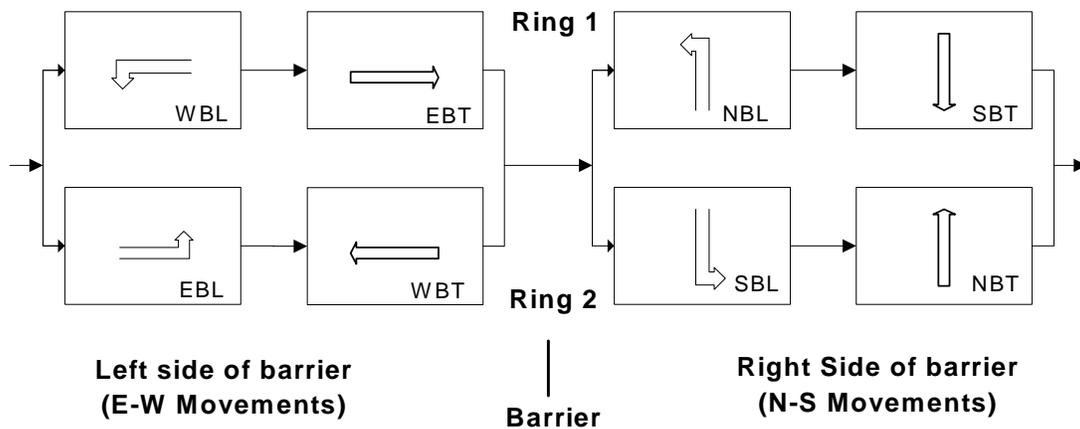
Figure 3. Dual-ring concurrent phasing scheme with assigned movements
