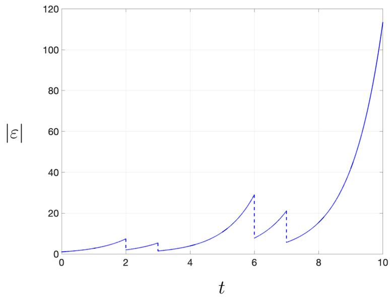
Figure 1.3: The evolution of the estimation error with respect to real time with the observer law that rejects delayed measurements. The vertical dashes represent the resets of  $\hat{z}$  according to  $\hat{z}^+$  in (1.4).
