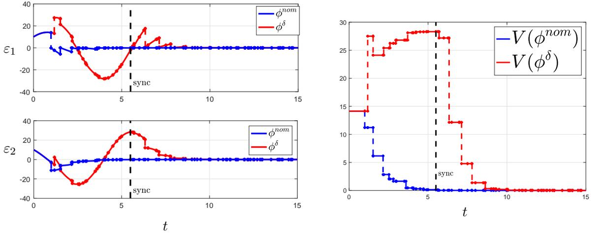
Figure 5.3: Plot of the error on the state components (left) and of  $V(x)$  evaluated along the trajectories of  $\phi^{nom}$  and  $\phi^\delta$  (right) for the case of initially mismatched clocks  $\tau_P$  and  $\tau_O$ .
