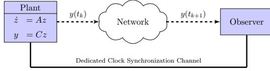
Figure 1.1: Block diagram of the networked plant-observer system.
