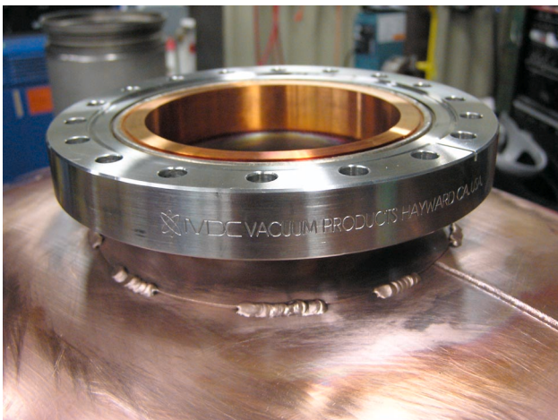
Figure 8. Port repaired by TIG welding.
