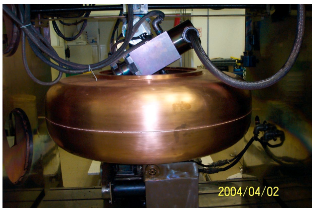
Figure 4. Inside cosmetic weld in the JLab e-beam welder.
