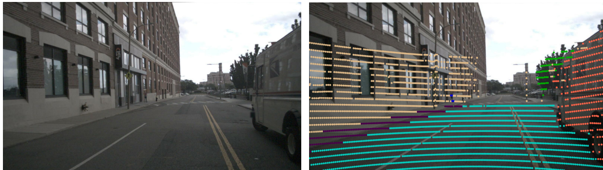
Figure 6.2: A benefit of querying a label is that we can retrieve corresponding sensor data of multiple types. Here, our algorithm finds both an RGB image and a segmented 3D LiDAR point cloud corresponding to a single label.
