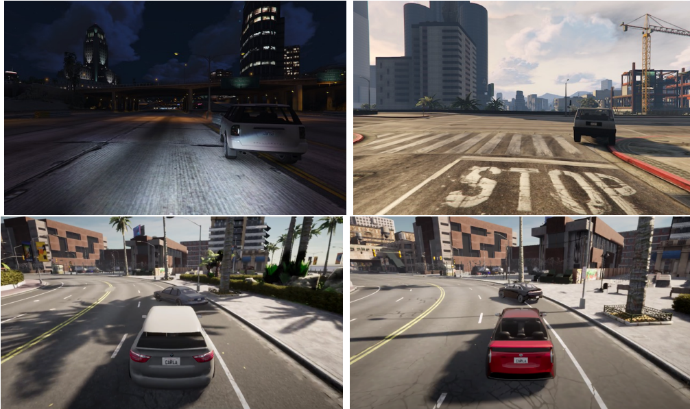
Figure 2.3: Scenes generated from the SCENIC program in Fig. 2.2 in GTA-V [63] (top images) and in CARLA [44] (bottom images) simulators
