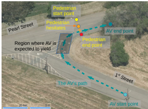
Figure 5.3: A bird's-eye view of the scenario S (left) and the (simplified) SCENIC program P_S encoding our test scenario.
