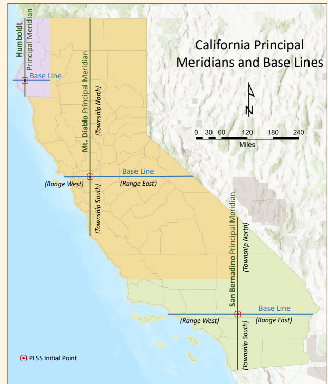
Figure S-1. Location of principal meridians, base lines, and initial points for the three U.S. Public Land Survey System surveys in California.
