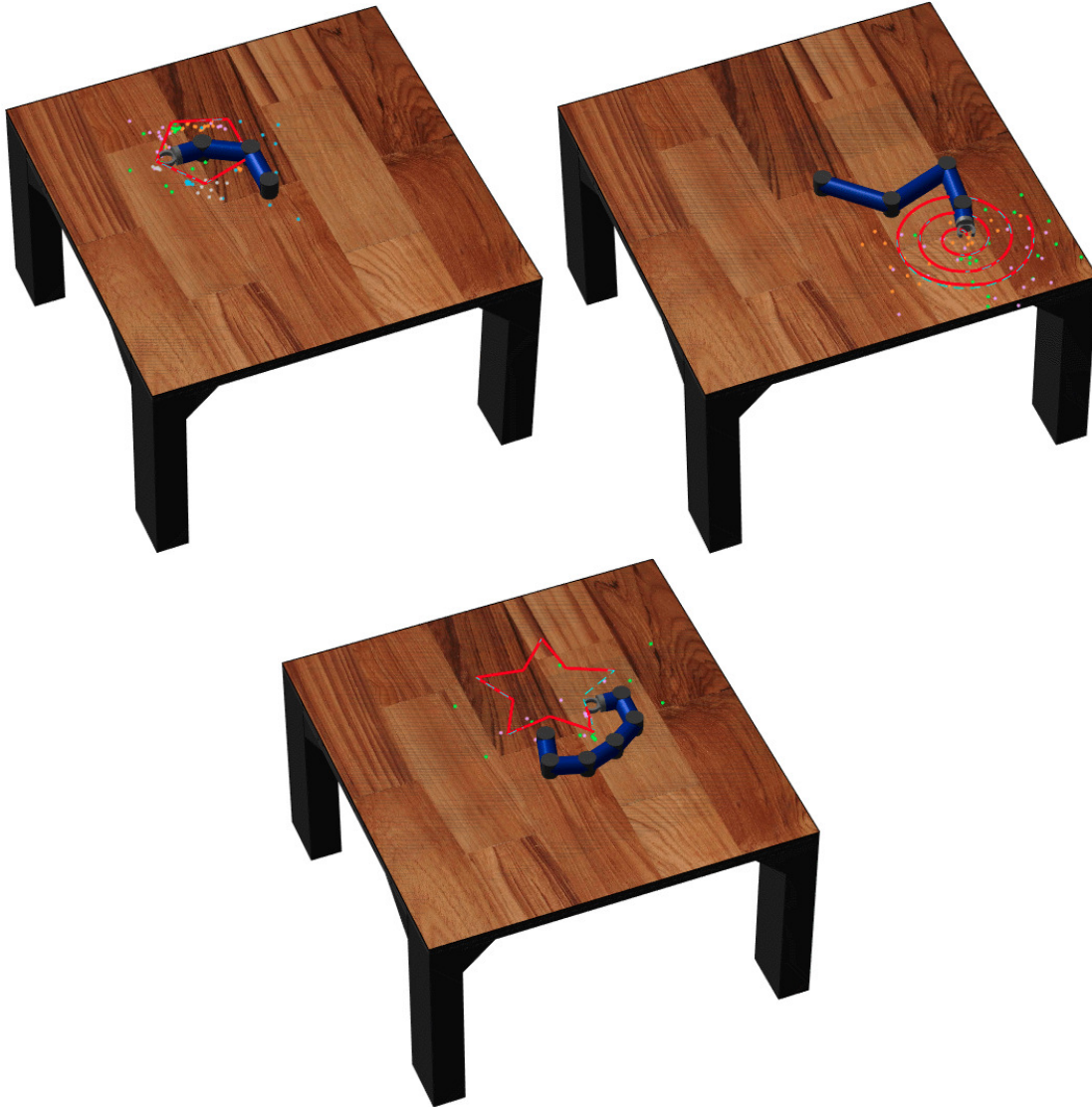
Figure 4.1: Images of a planar 3, 4, 6 DOF manipulator arm recreating a pentagon, spiral, and star trajectory from simulated teleoperation test points. The colored dots on the image (green, and pink), represent locations of the support points optimized from the SOLAR_GP.
