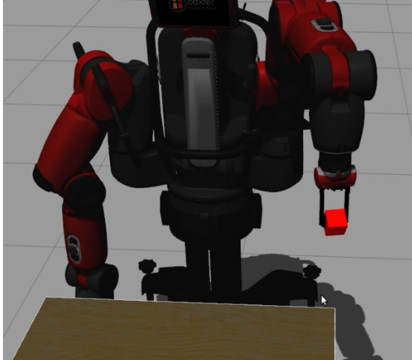
Figure 4.6: Image of Baxter robot during a teleoperation experiment to pick up a block from a table
