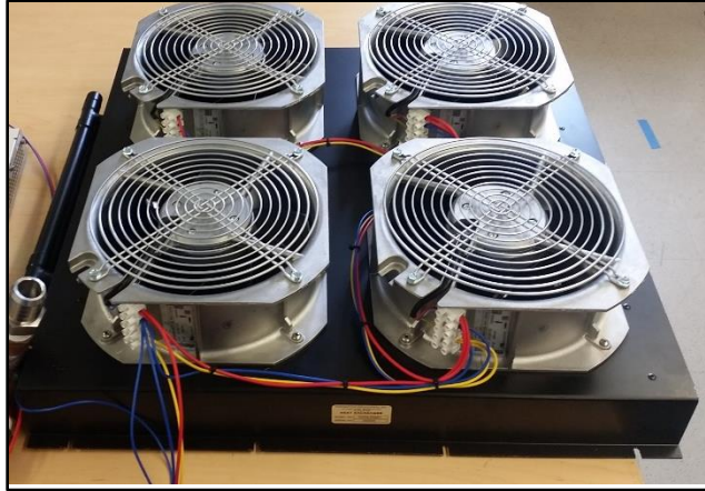
Figure 53: heat exchanger cooling fans
