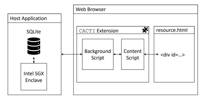
Figure 5.6: Overview of CACTI client-side components.
