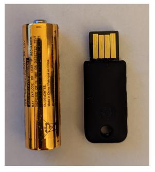
Figure 6.5: Solokey token compared to a standard AA battery.
