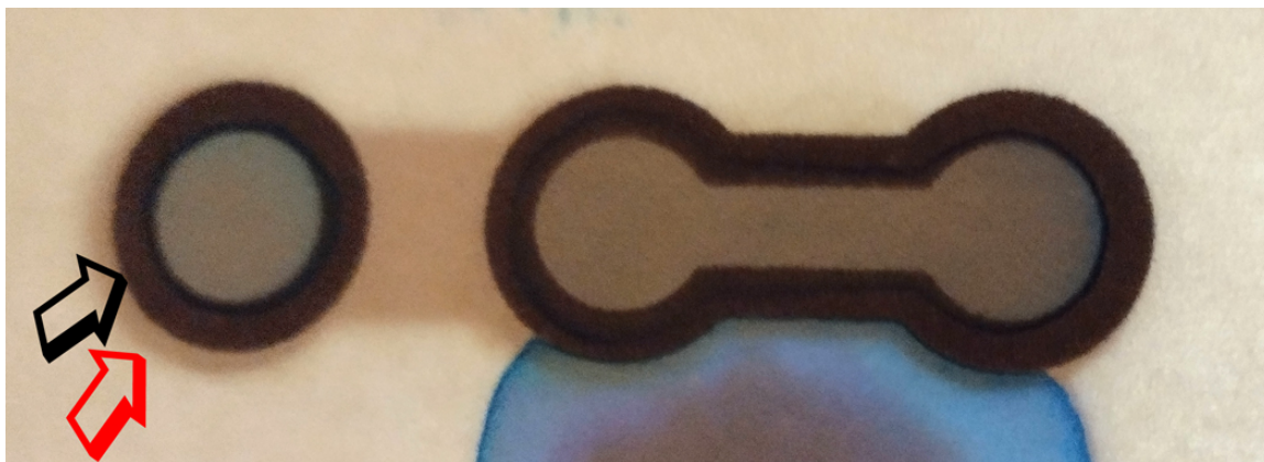
Figure 8.4: In this multilayer paper microfluidic device fabricated using adhesive A, one layer was misaligned during assembly, which led to a loss of fluid containment between the layers. The red and black arrows indicate the shift from proper alignment.
