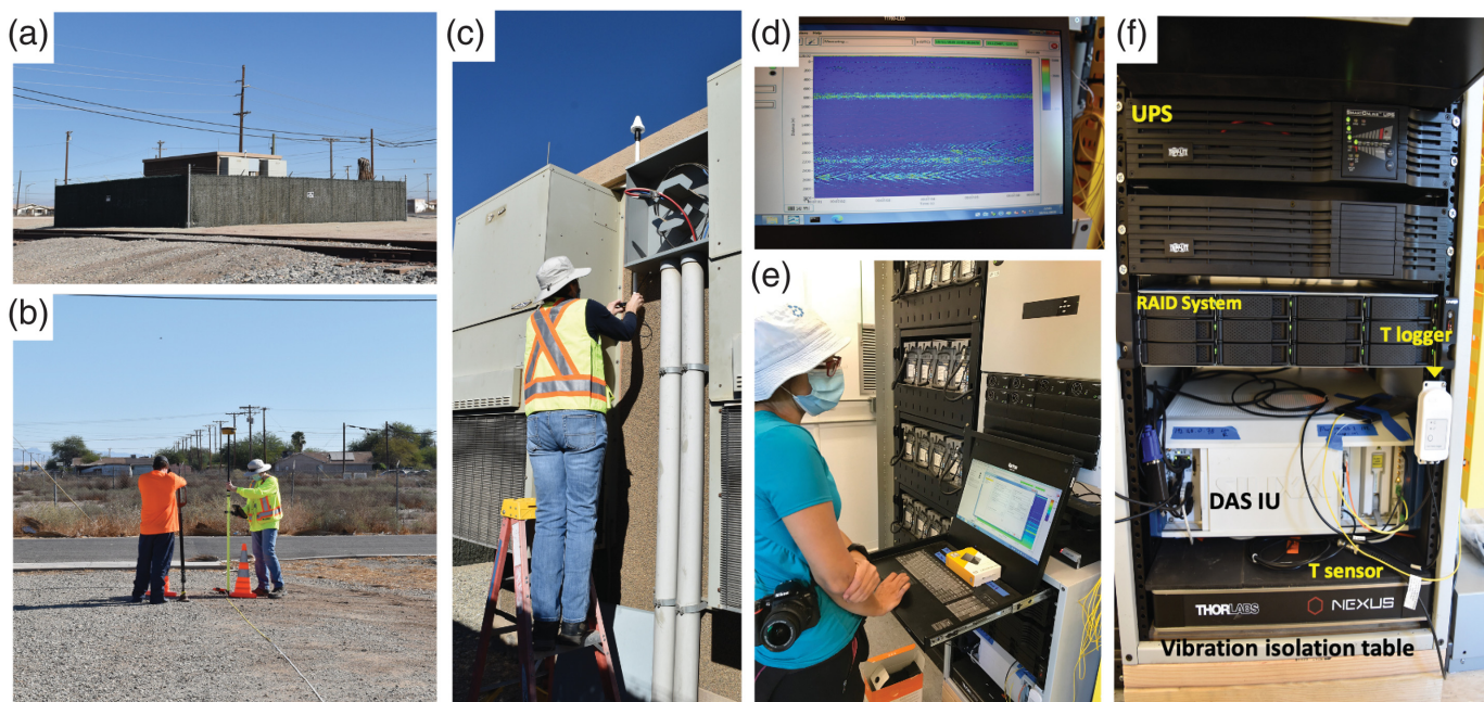
Figure 2. Field installation and system montage. (a,b) the Calipatria, California, intermediate light amplification (ILA) hut and a tap test location, respectively; (c) installation of the Global Positioning System antenna and external environmental monitoring sensor; (d–f) the first recorded data, interrogator unit (IU) configuration process, and IU monitoring system stack, respectively. UPS, uninterruptible power supply.
