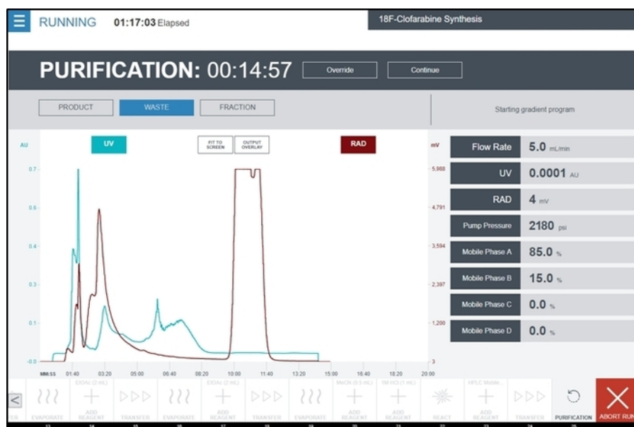
Figure 9: Screenshot of the radiosynthesizer user interface while running the Purification unit operation during the synthesis of [ 18 F]CFA. The UV detector and radiation detector outputs of the purification/formulation module are displayed on the central graph in real time. Additional feedback from the detectors and HPLC pump are shown on the right side of the screen. The operator collects the product peak by temporarily selecting Product when the peak begins to appear and then switching back to Waste after the complete peak has been seen. Please click here to view a larger version of this figure.
