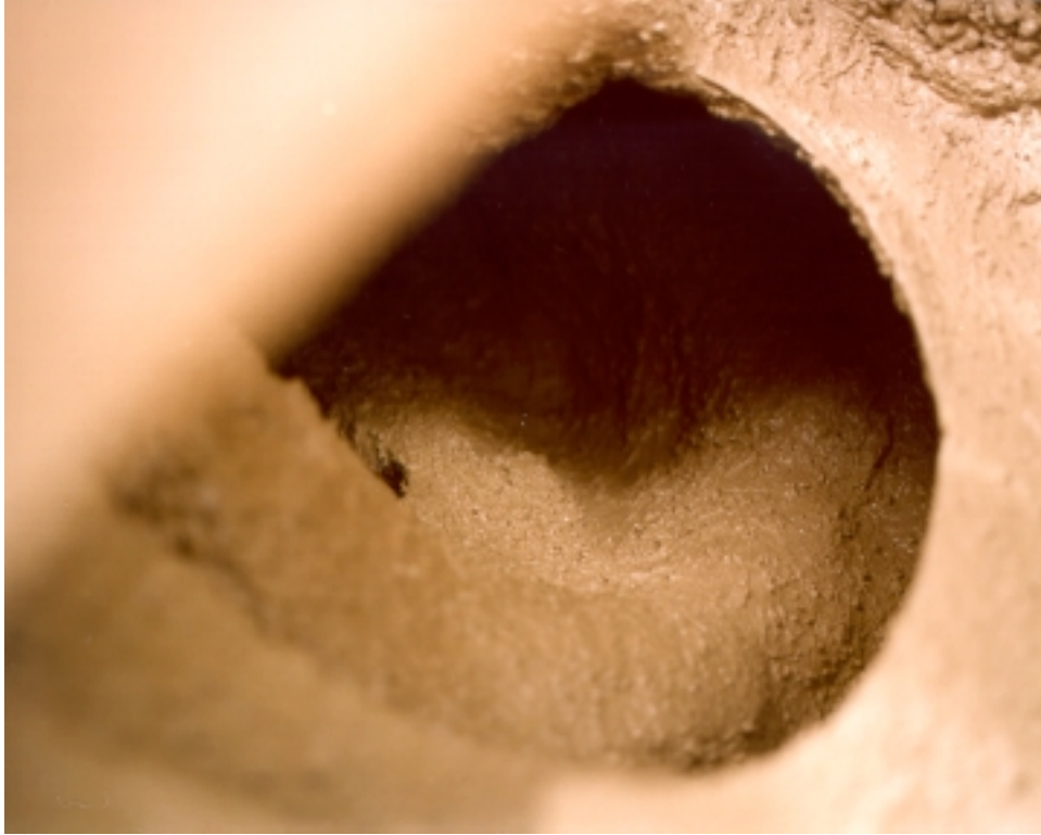
Figure 8.3. Clogged Fins inside Ready Mix Truck, North Tangent.
