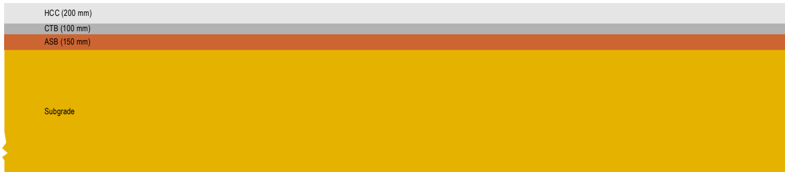
Cross-section View of Test Area (1:300 scale)
