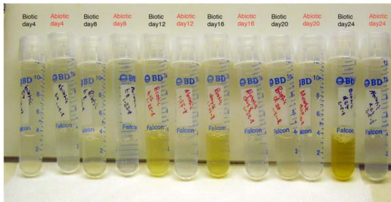
Figure 6.9: Centrifuged fractions of all samples from day 4-24. Compared to the abiotic and abiotic/amonabactin set-up the biotic samples show a yellow color of the supernatant that intensifies with time.
